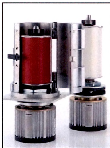
Fig. 2.21 Spindle assemblies showing individual drive and integrated bearing
