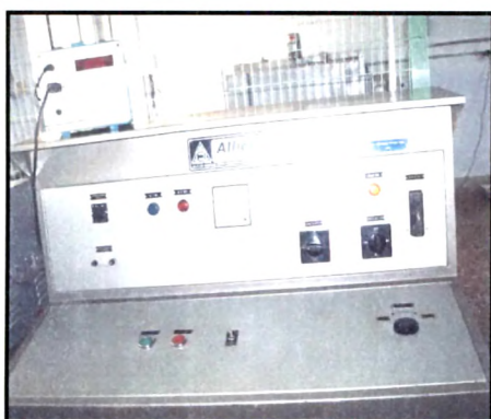
Fig. 4.12 Set up for measuring dielectric strength
