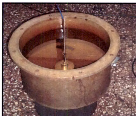
Fig. 4.12 Set up for measuring dielectric strength
