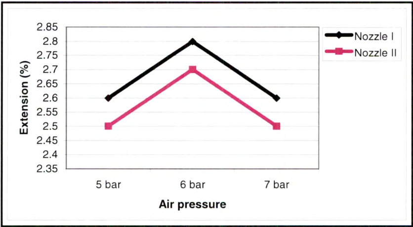
Fig. 6.6(b) Effect of air pressure on hybrid yarn extension at 1% overfeed
