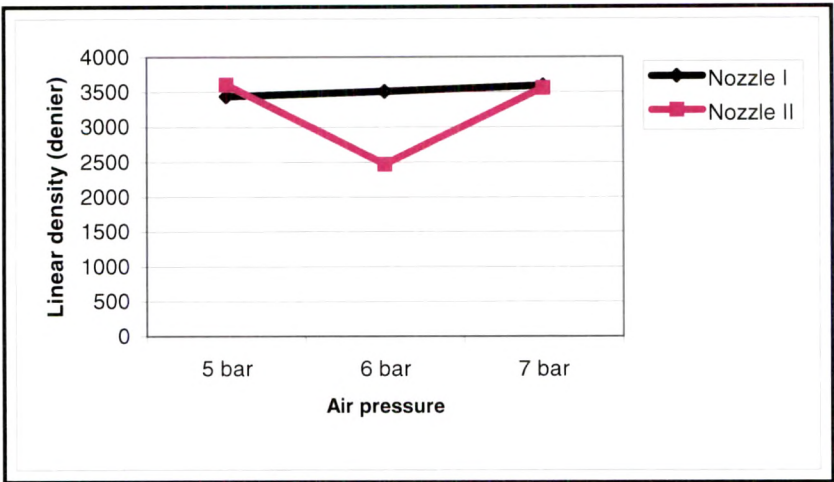
Fig. 6.4 (b) Effect of air pressure on hybrid yarn linear density at 1% overfeed
