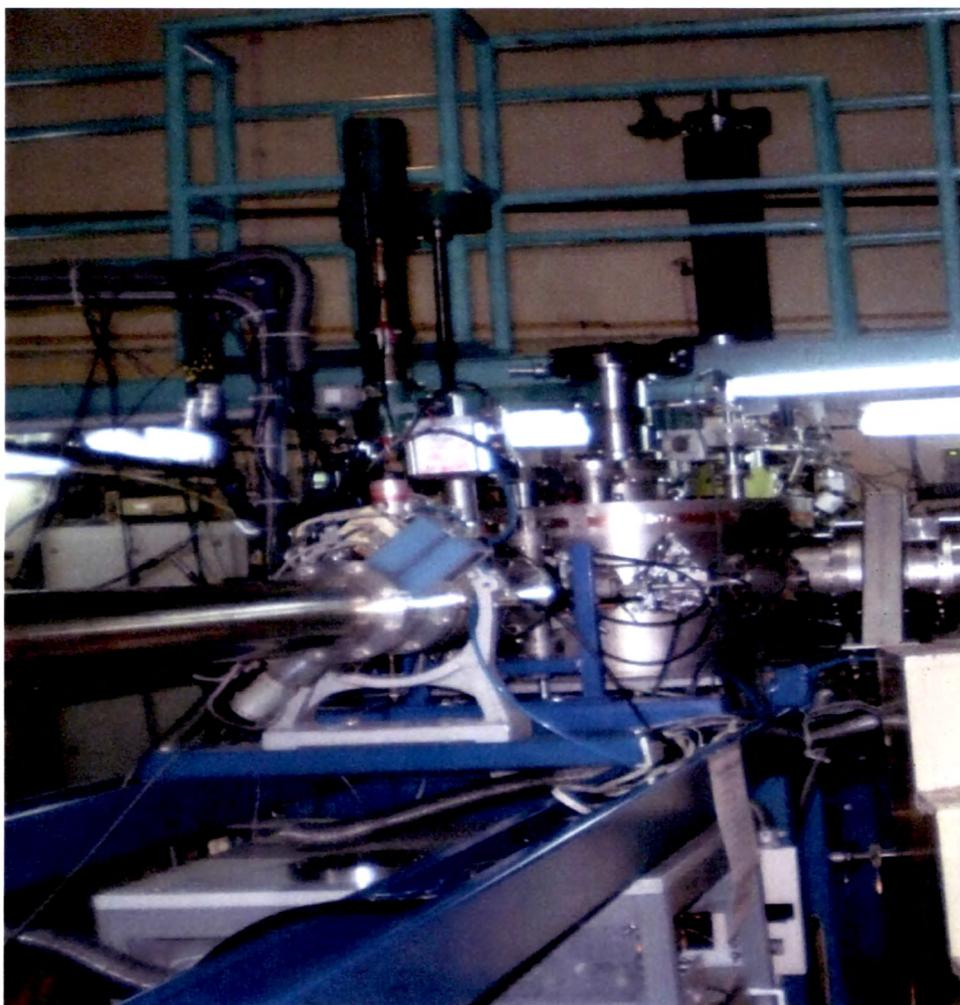
**Fig. 2.2 Material science chamber for irradiation at IUAC New Delhi.**
