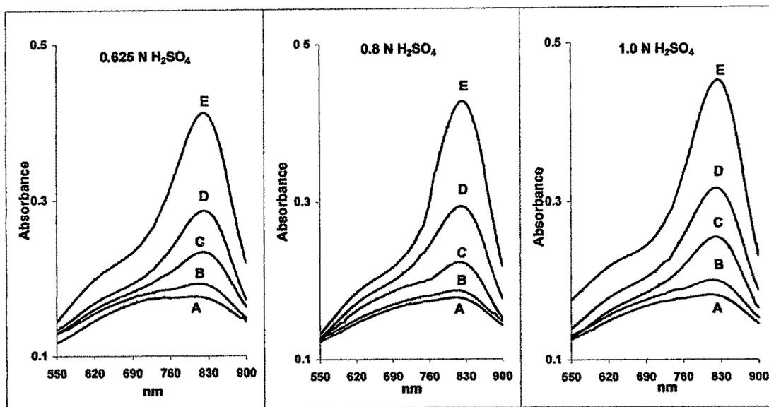
**Figure 1.** Time course of color development in Pi assay. Color was developed using 4  $\mu\text{g}$  Pi. Concentrations of  $\text{H}_2\text{SO}_4$  were 0.625 N, 0.8 N and 1.0 N. Optical density measurements at 660 nm and at 820 nm were made at specified time periods as indicated. Each data point represents average of 3 independent observations. Variation ranged from 2-3 %.
