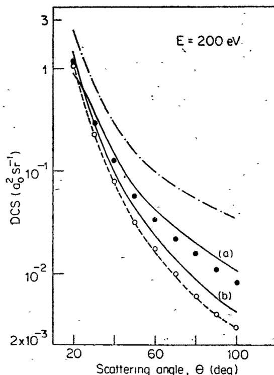
Figure 1. Differential scattering cross-sections for the elastic scattering of electrons from H(2S) at 200 eV. Solid curve a.—present calculations, broken curve—present calculation in the Glauber approximation. Solid curve b—data of Pundir *et al* (1982), dash—dot curve HHOB results (Rao and Desai 1983). + — EBS results (Joachain *et al* 1977). — — OM results (Joachain and Winters 1980).
