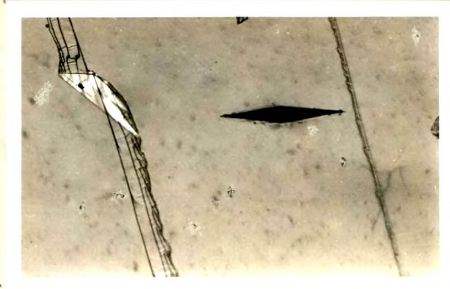
Fig. 5.9 (a,b) show the photomicrographs of indentation marks produced by Vickers and Knoop indenters on cleavage counterparts of melt grown sodium nitrate crystal.
