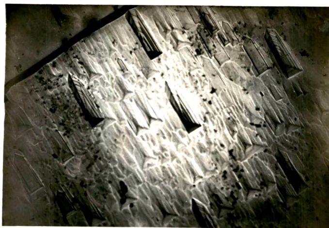
Fig. 11.3a (x 45) photomicrograph of dislocation etch pits by etching the freshly cleaved surface of calcite in 60% acetic acid for 3 min at 75°C.
