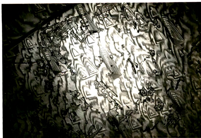
Fig. 11.3b (x 45) MBI interferogram of the surface shown in fig. 11.3a.
