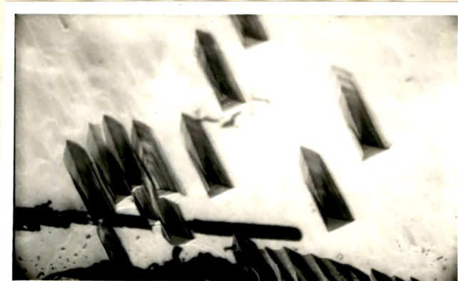
Fig. 11.2a (x 95) photomicrograph of dislocation etch pits by etching the freshly cleaved surface of calcite in 60% acetic acid for 3 min at 62.5°C.
