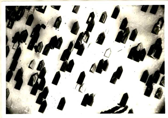
Fig. 11.1a (x 95) photomicrograph of a dislocation etch pits by etching the freshly cleaved surface of calcite in 60% acetic acid for 3 min at 43°C.
