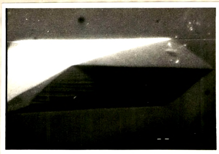
Fig. 11.8 (x 1720) (SEM) electron micrograph of an etch pit on a calcite cleavage etched for 4.5 min. by 60% glacial acetic acid at 40°C.
