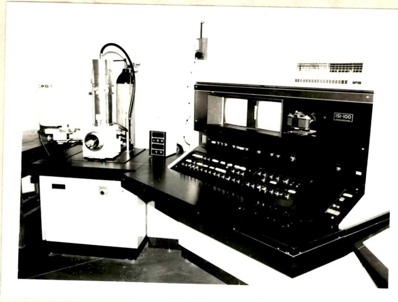
Fig. 2.10 ISI Scanning Electron Microscope.
