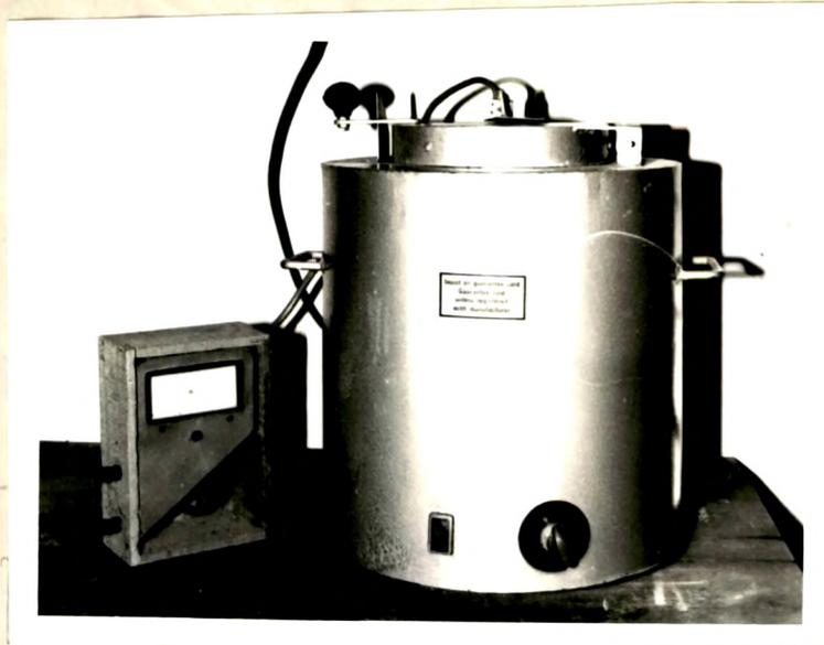
Fig. 2.13 Vertical temperature gradient crucible furnace.
