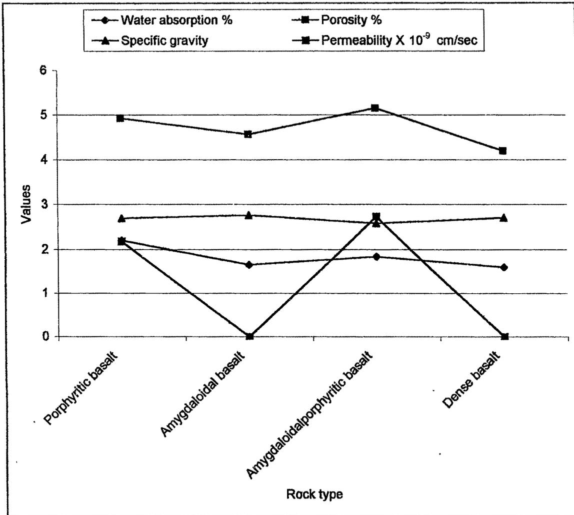
Fig. 13: Physical properties of foundation rocks, Karjan dam
