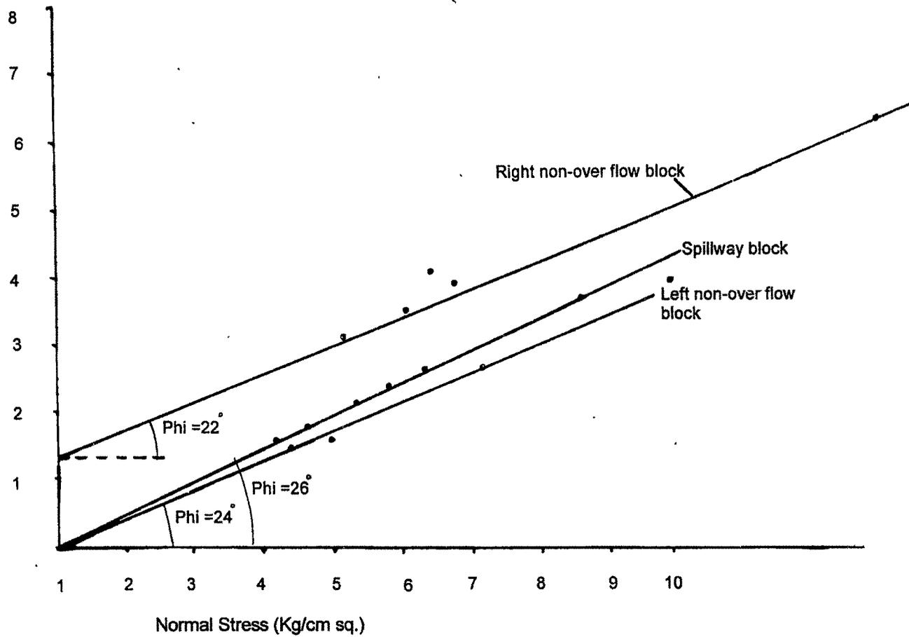
Fig. 15: Plot of in-situ shear tests on weathered rock seams at Karjan dam foundation
