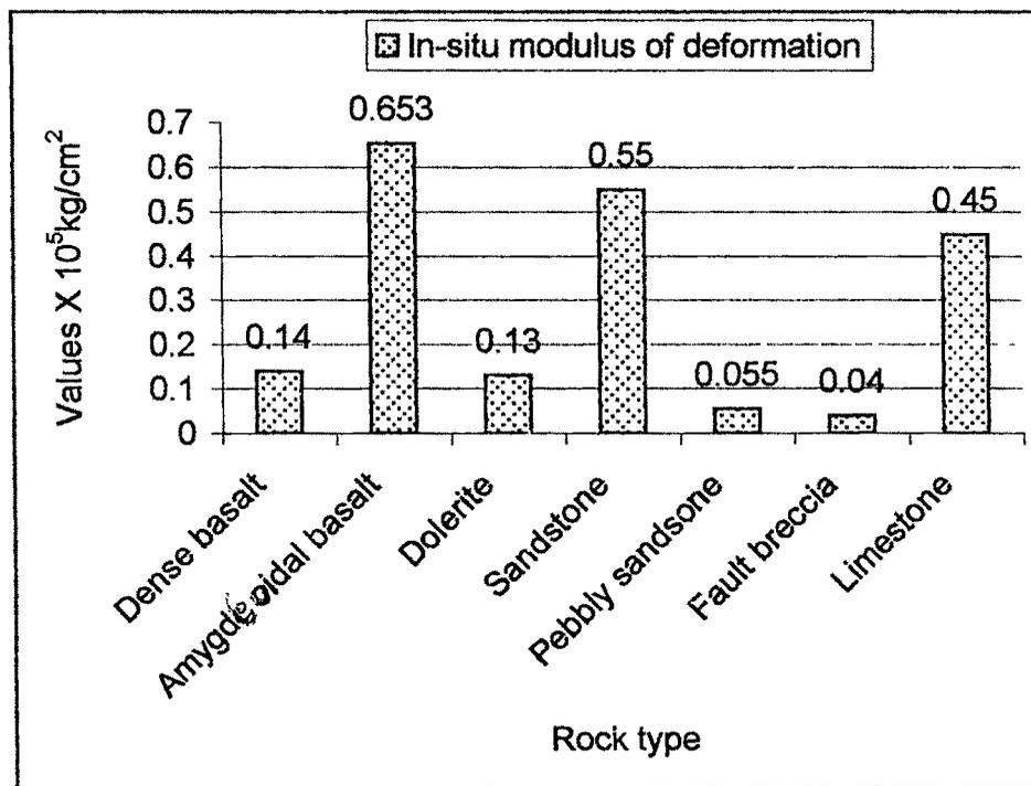
(b) Modulus of deformation of rock mass
