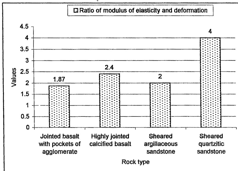
(b) Ratio of modulus of elasticity and deformation of foundation rocks
