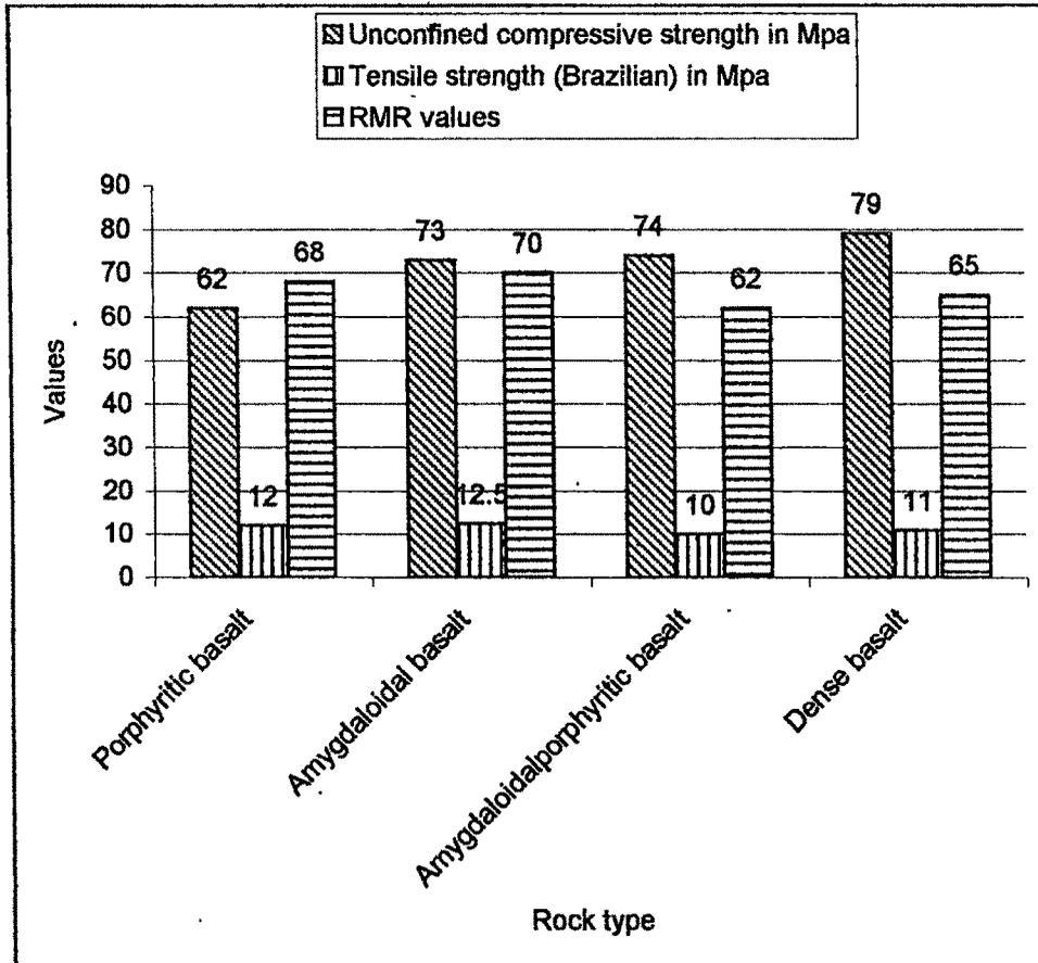
Fig. 14: Compressive, tensile strength and rock mass rating of foundation rocks, Karjan dam
