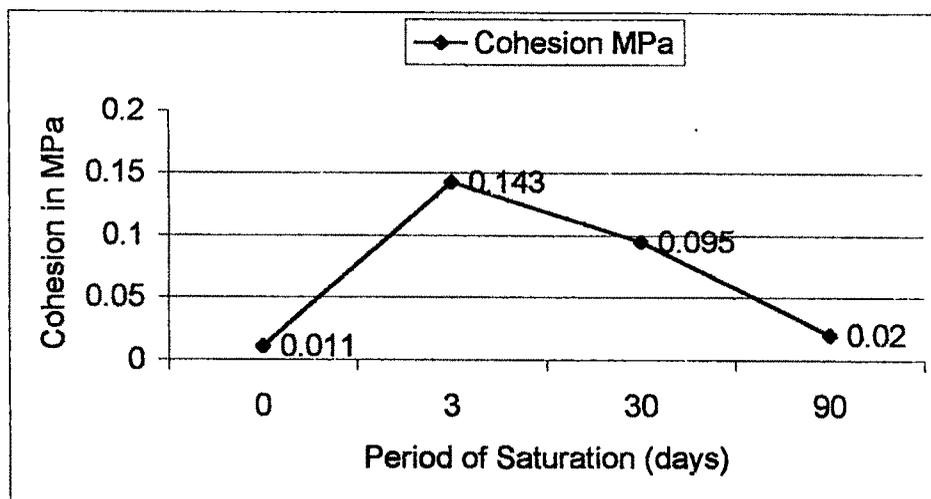
Fig. 12: Shear parameters of chlorite coated joints in the dolerite rock based on the laboratory tests, Sardar Sarovar (Narmada) Project
