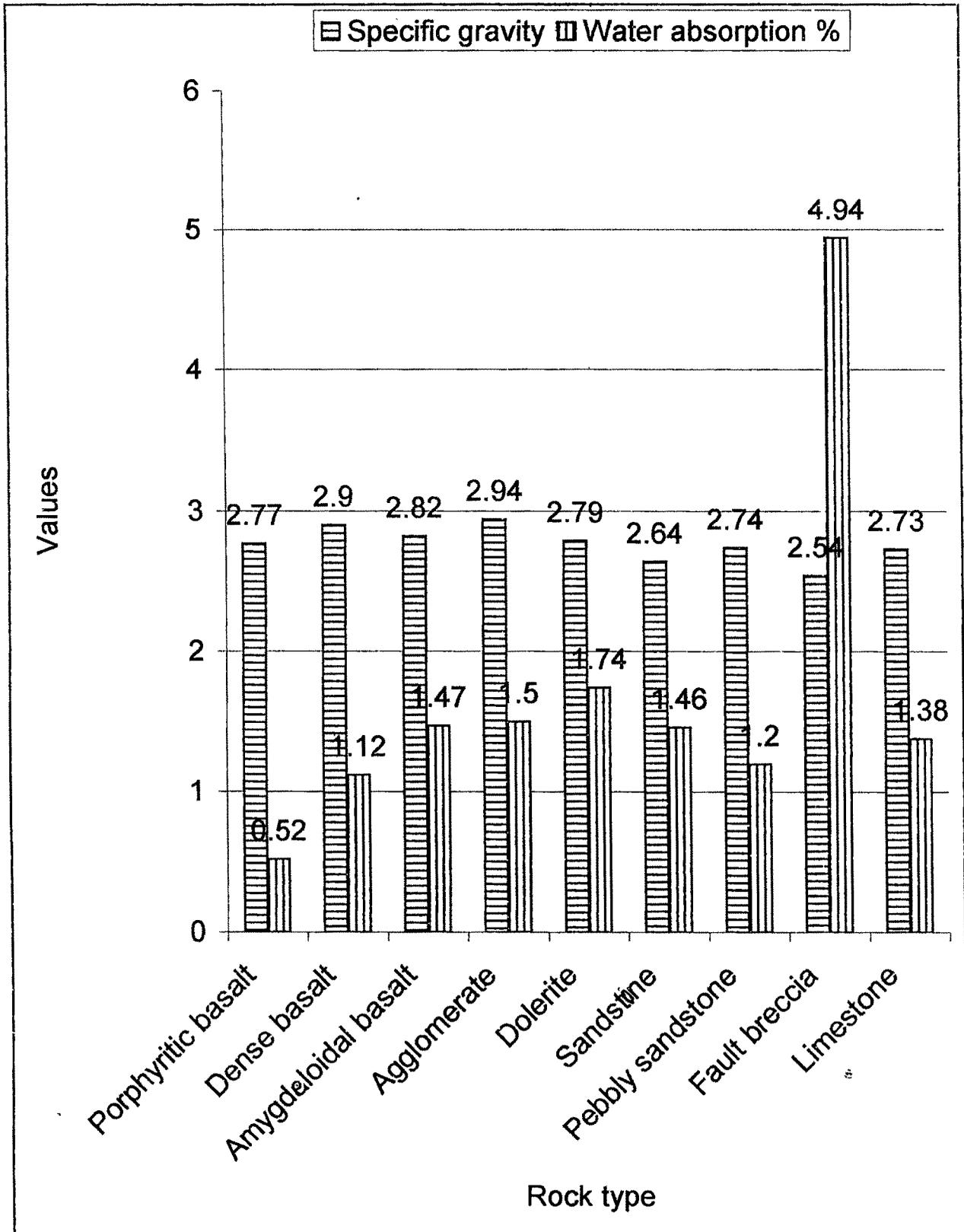
Fig. 7: Specific gravity and water absorption of the foundation rocks, Sardar Sarovar (Narmada) Project
