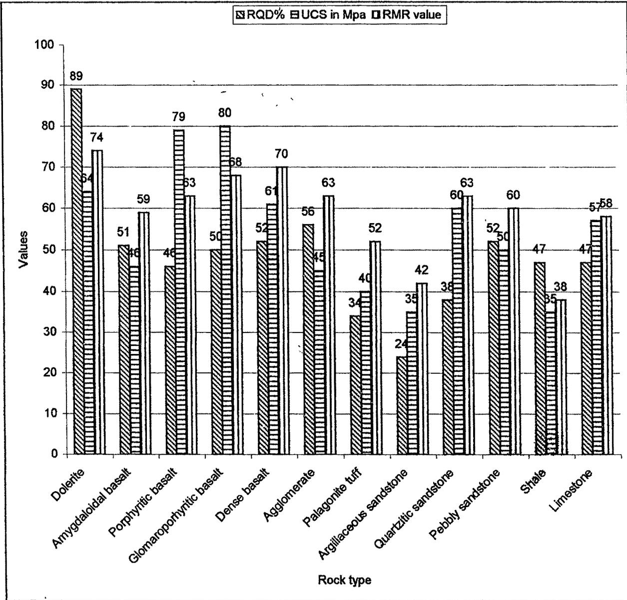
Fig. 11: Rock Quality Designation, Compressive strength and Rock Mass Rating of main dam foundation rocks, Sardar Sarovar (Narmada) Project
