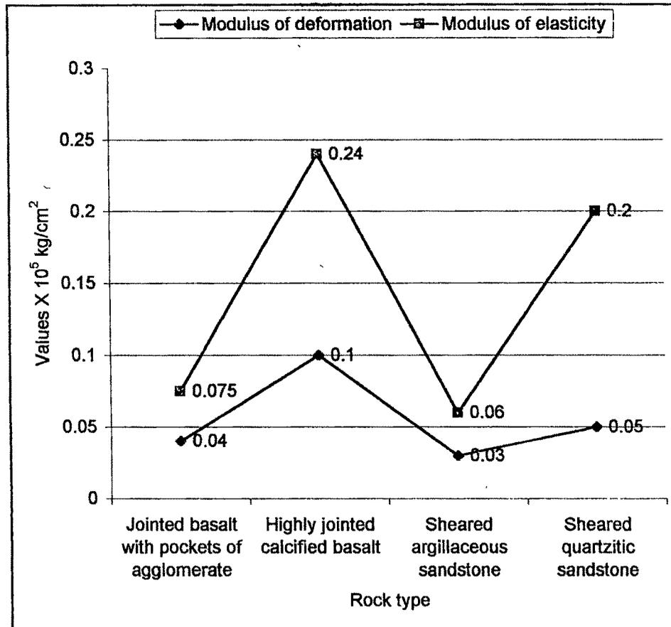
(a) Modulus of deformation and modulus of elasticity of foundation rocks
