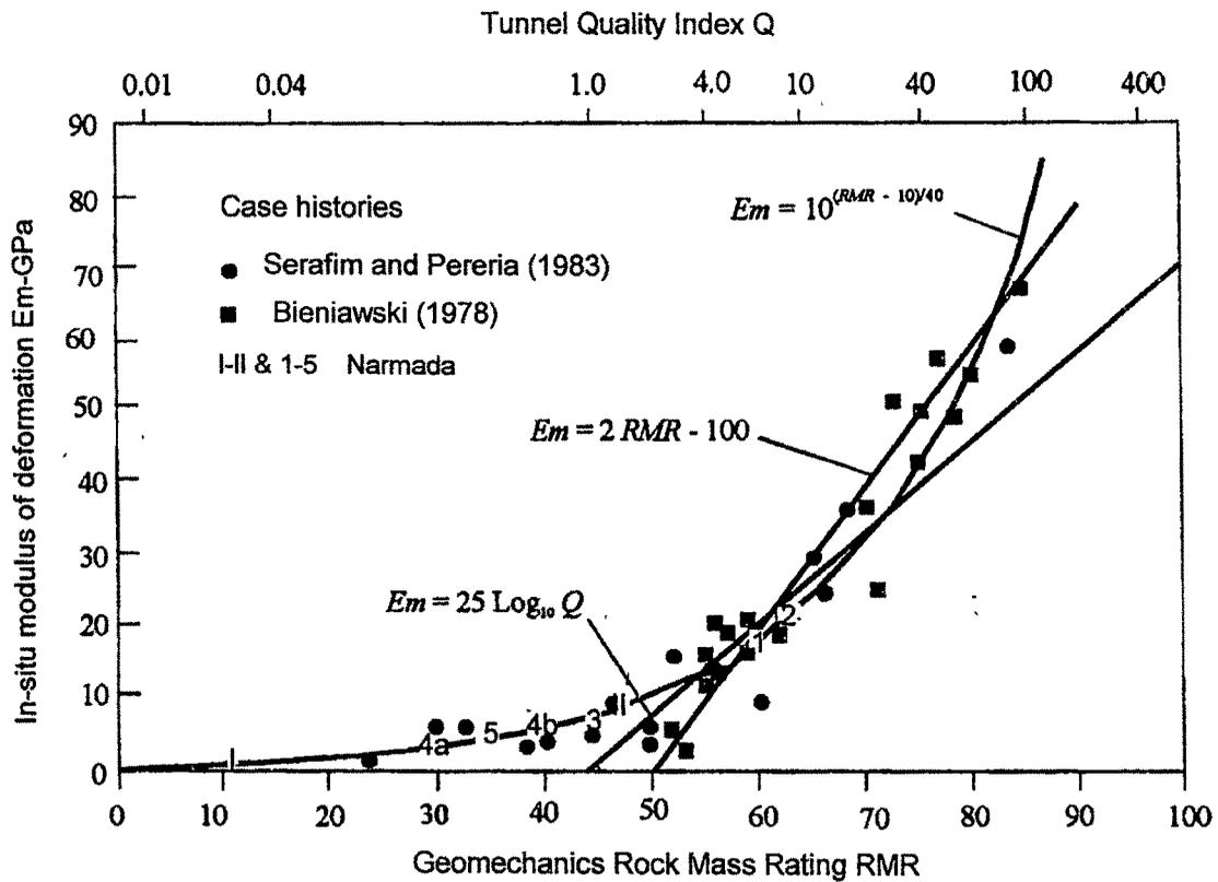
Fig. 5: Prediction of in-situ deformation modulus  $E_m$  from rock mass classification (After Hoek et. al. 1997)
