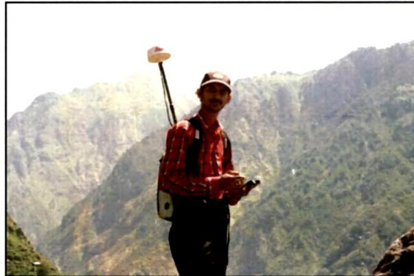
**Plate II.2 - Use of Leica GS5 GIS-GPS data collection system for inventory of field data**
