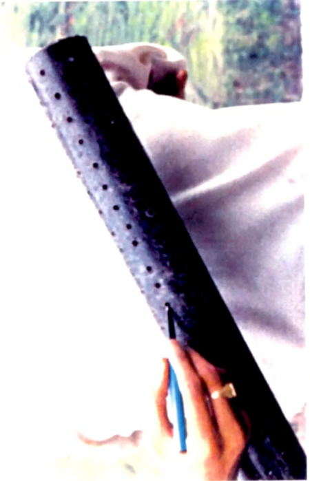
B. Making of 3mm \Phi Perforation in PVC Pipe
