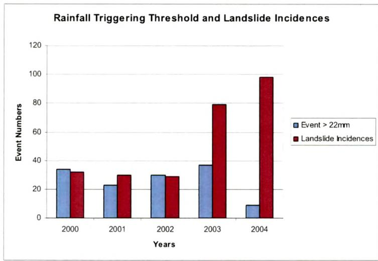
**Figure 6.3 - Correlations of Rainfall Triggering Threshold and Landslide Incidences, Mangti Landslide Environ.**
