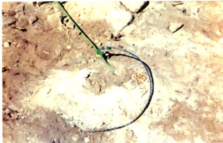
**C.** Field photograph of completely filled blast hole with explosives, connected in network with a detonator
