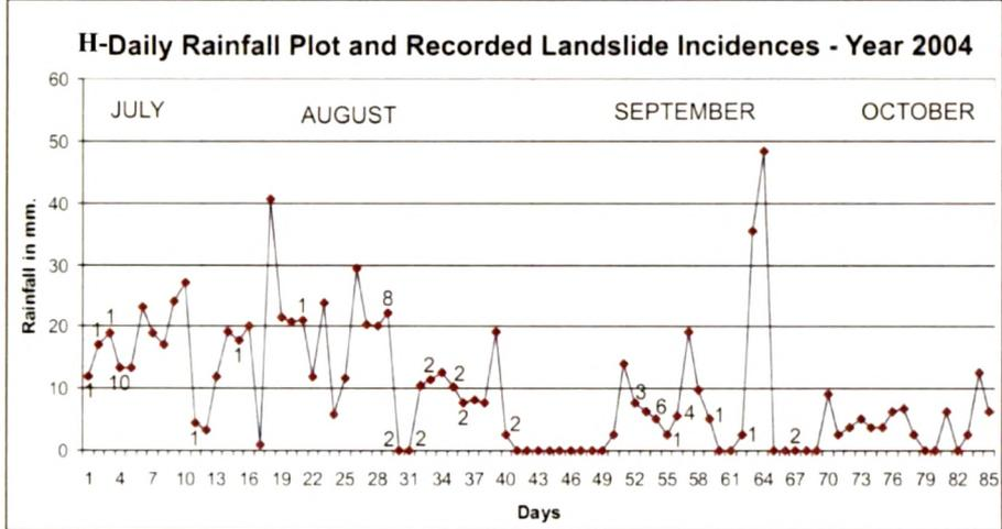
**Figure 6.2 - Correlations of Observed Rainfall Hydrographs and Landslide Incidences, Mangti Landslide Environ**
