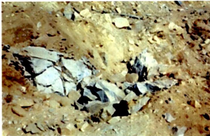
**E.** Field photograph of the fractured rock mass after carrying out uncontrolled blasting during construction phase of last 1km stretch of TJRC beyond Galagad village towards Jipti
