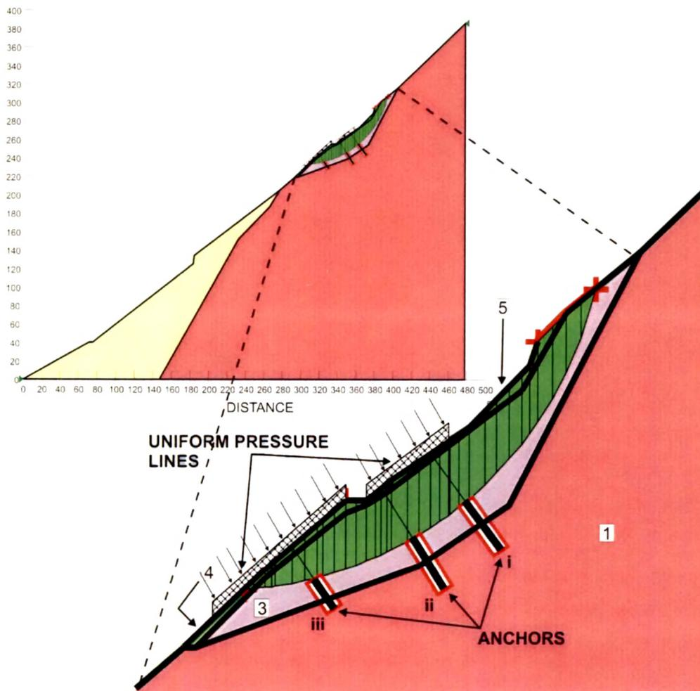
Figure 7.5a – 2-D GeoSlope Slope Stability Model of Upper Level-Mangti Landslide
