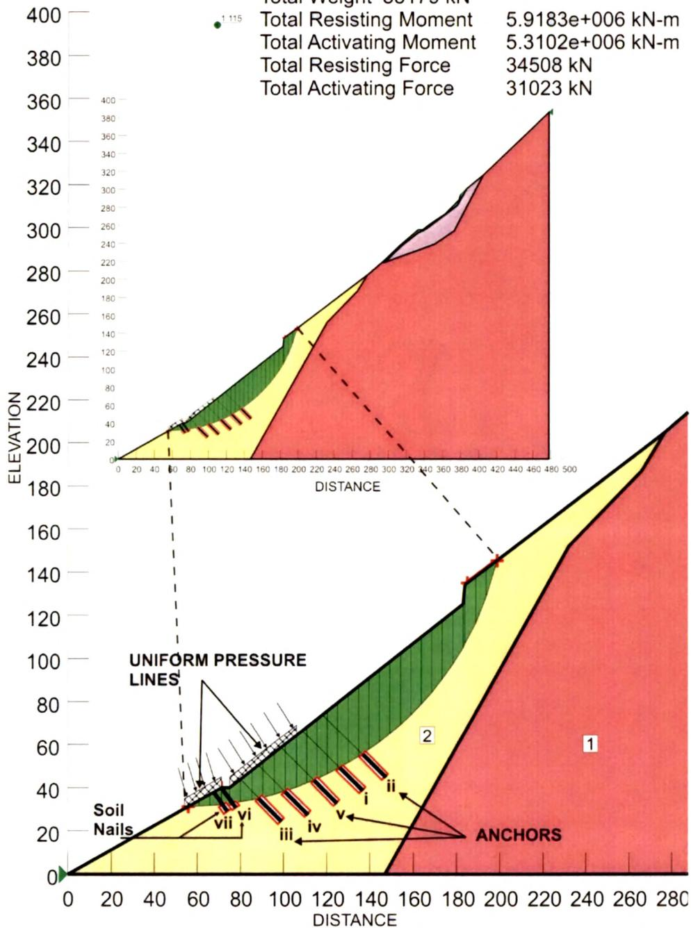
**Figure 7.5b – 2-D GeoSlope Slope Stability Model of Lower Level-Mangti Landslide**
