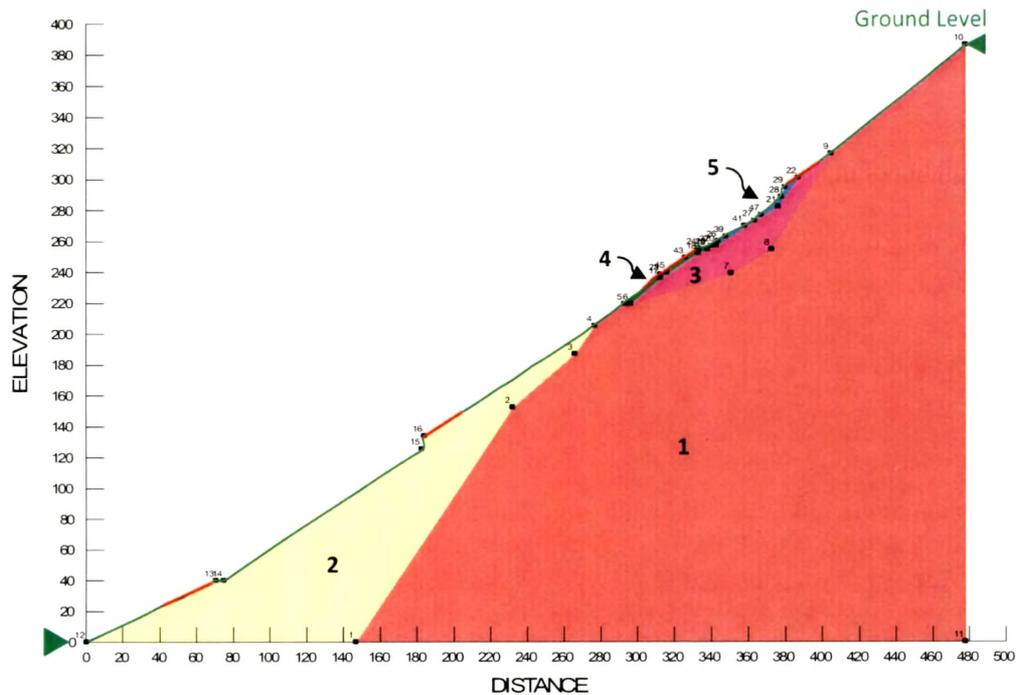
**Figure 7.2 – 2-D GeoSlope Model of Mangti Landslide Showing Typical Regions for Slope Stability Analysis**
