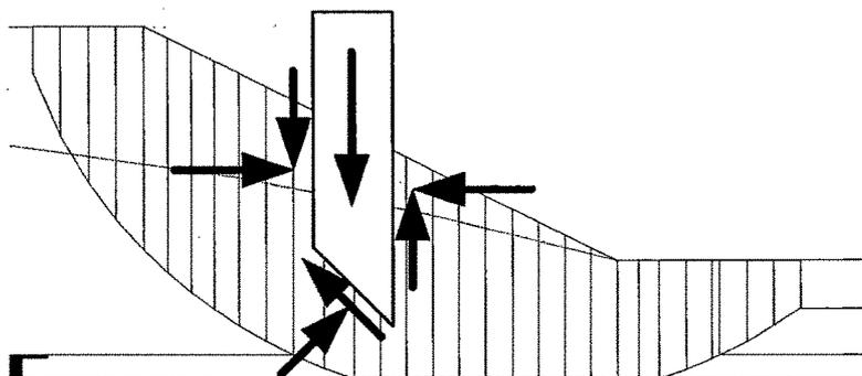
Figure 7.1 – Slice Discretization and Slice Forces in a Sliding Mass
