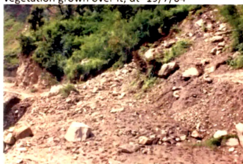
26c. The slope mass is seen to be completely saturated and the soil is flowing down the slope like a viscous fluid. Although the traveling rate is too low, about 5cm/min; dt-29/7/04
