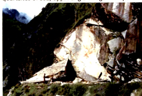
13. View of planar rockslide occurred in quartzites at the contact zone of MCT; dt-4/7/04
