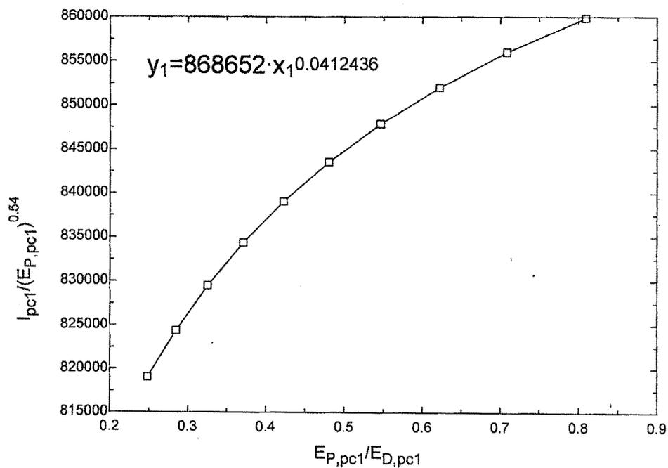
**Fig. 5.17 Plot of TCI v/s Exergetic Efficiency for Pre-cooler-1**
