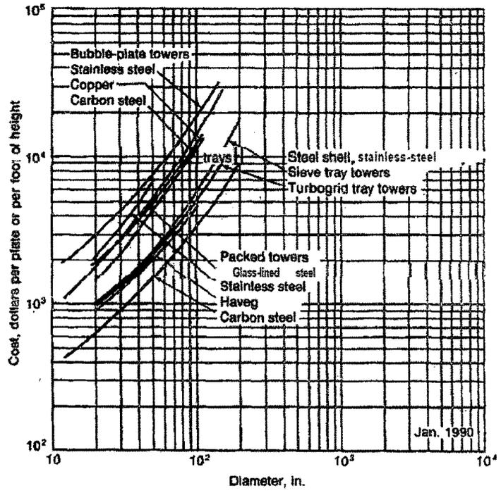
Fig. 5.4 Cost of Tower Including Installation [158]
