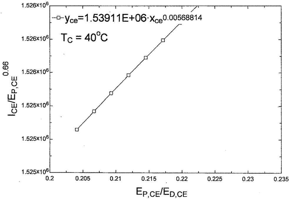
Fig. 5.11 Plot of TCI v/s Exergetic Efficiency for C-E Assembly for  $T_a = T_c = 40^\circ\text{C}$
