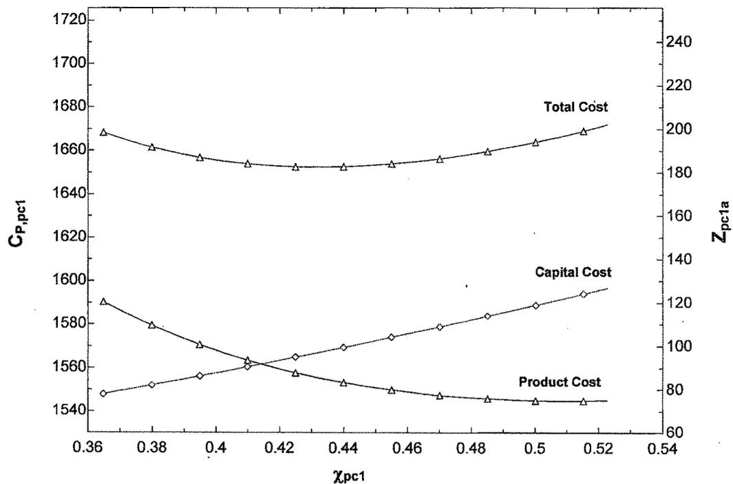
**Fig. 5.19 Optimum Product Cost for Pre-cooler-1**
