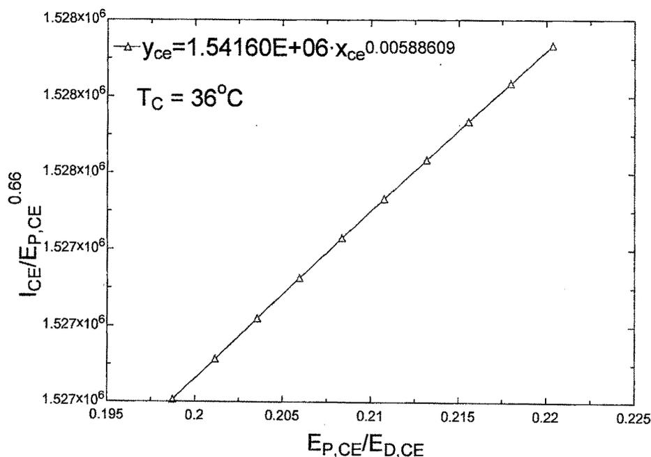
**Fig. 5.9 Plot of TCI v/s Exergetic Efficiency for C-E Assembly for  $T_a = T_c = 36^\circ\text{C}$**
