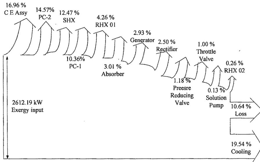
**Fig. 5.2 Rate of Exergy Destruction of Various Components**
