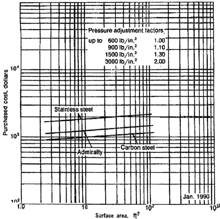
Fig. 5.7 Cost of Double Pipe Heat Exchanger [158]
