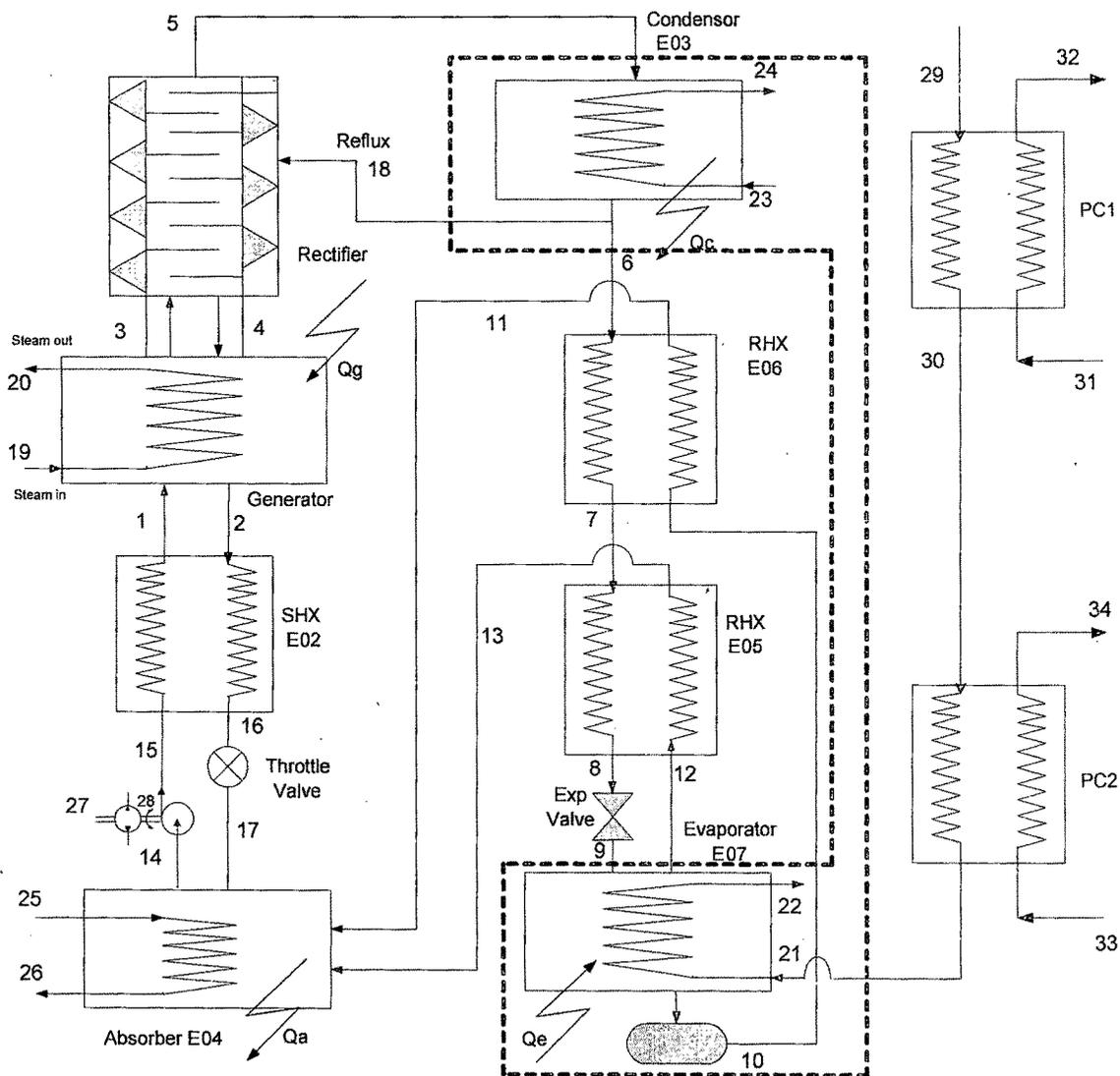
**Fig. 5.1 Sub systems of AAVAR System for Exergoeconomic Optimization**
