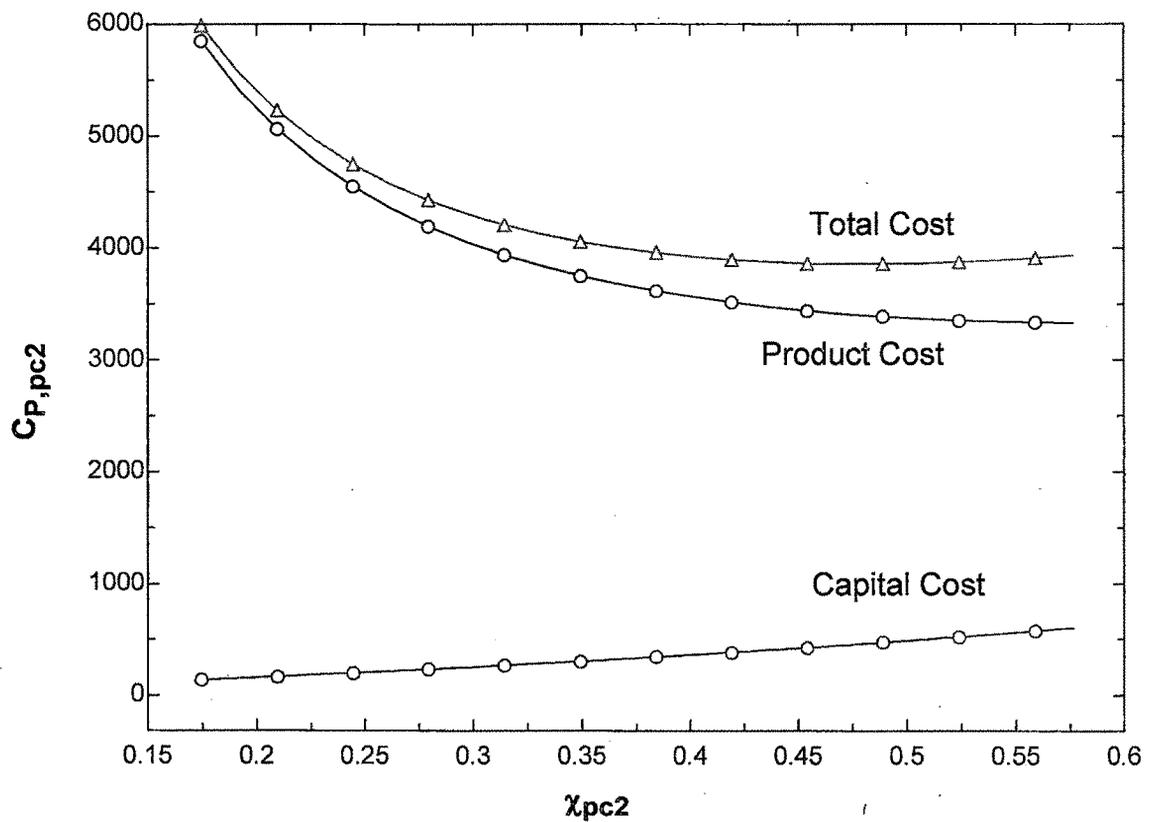
**Fig. 5.20 Optimum Product Cost for Pre-cooler-2**
