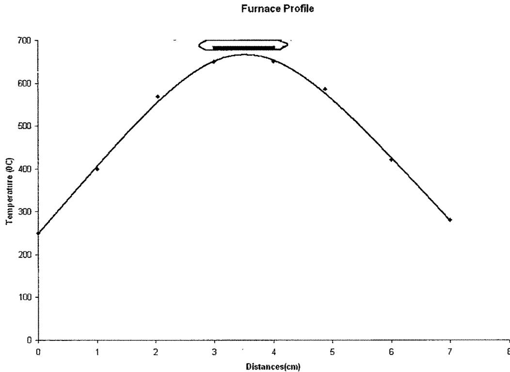
**Figure- 1 Profile of furnace ( Temperature gradient  $65$   $^{\circ}\text{C}/\text{cm}$ )**
