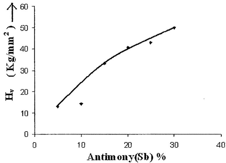
Figure- 8 Vicker's Hardness  $\rightarrow$  Sb%
