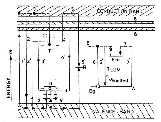
•-ELECTRON, O-HOLE, T-ELECTRON TRAP, H-HOLE TRAP Eg-GROUND STATE OF IMPURITY A, R-RECOMBINATION SITE E - EXCITED STATE OF IMPURITY A, -----EXCITED STATE Em-METASTABLE STATE OF IMPURITY A
