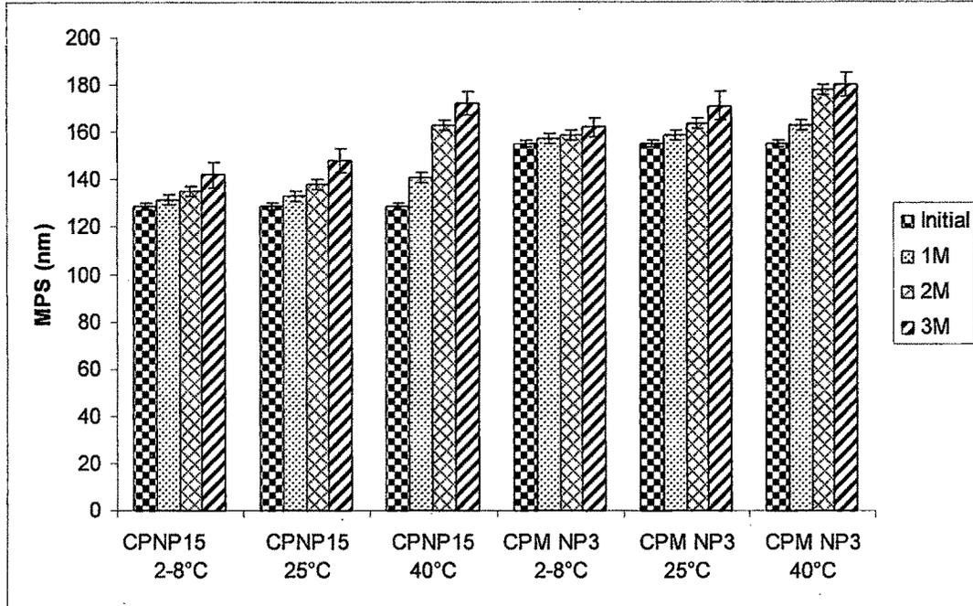
**Fig. 5.17: Effect of storage at 2-8°C, 25°C and 40°C on Mean Particle Size (MPS) of Lyophilized Cytarabine loaded PLGA NP (CPNP15) and Cytarabine loaded PLGA-mPEG NP (CPM NP3). The values are mean of three batches with  $\pm$  S.D**
