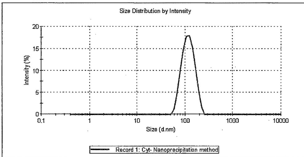
Fig. 5.5: Size distribution graph of Cytarabine loaded PLGA NP batch No. CPNP15
