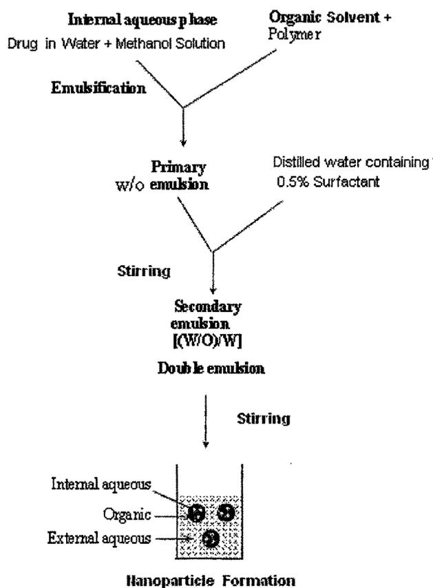
Fig. 5.1: Flow diagram for formulation of NP
