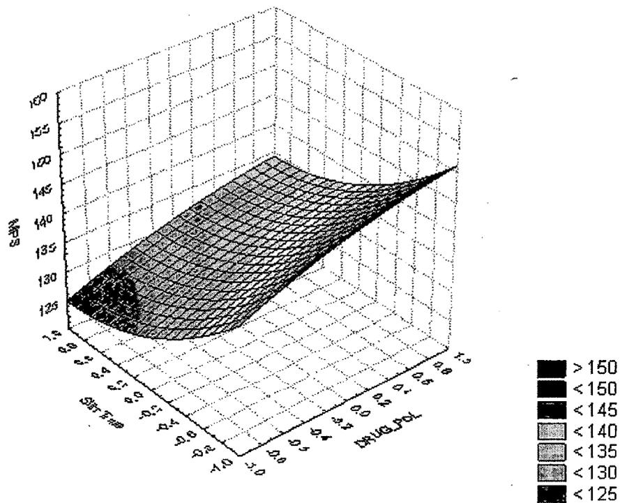
Fig. 5.3b: Surface response plot for MPS against X1(drug: polymer ratio) and X2 (stirring time) values ranging from -1 to +1.
