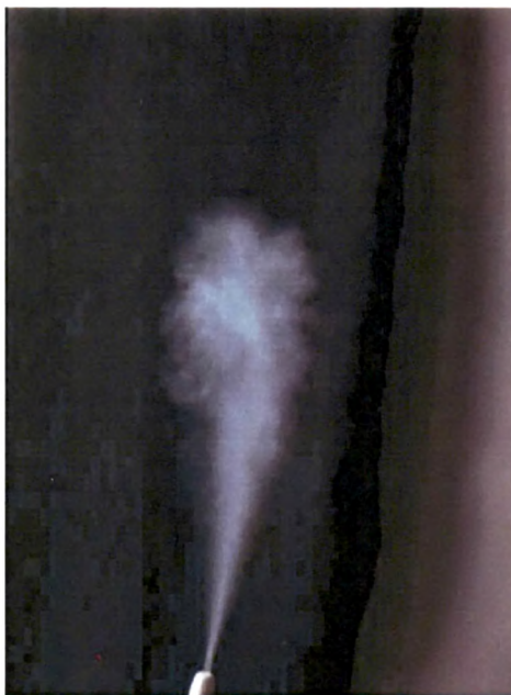
Fig. 8.4 The spray pattern (shape) of CRV loaded alginate microspheres from MIAT ® nasal monodose insufflator.
