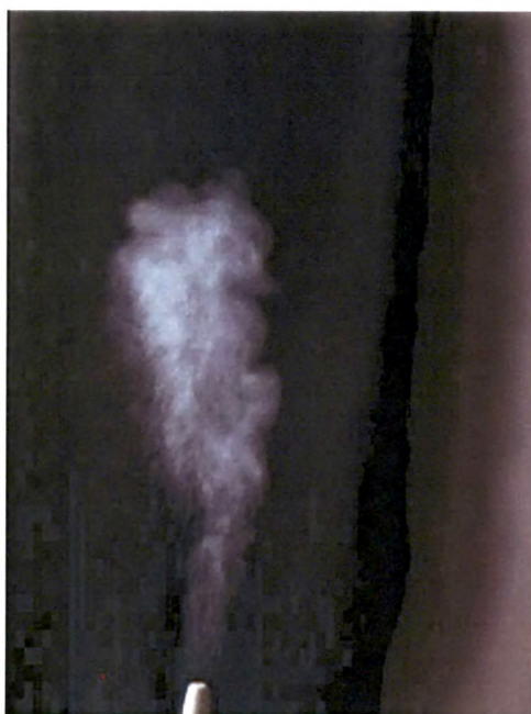
Fig. 8.5 The spray pattern (shape) of NTD loaded alginate microspheres from MIAT ® nasal monodose insufflator.
