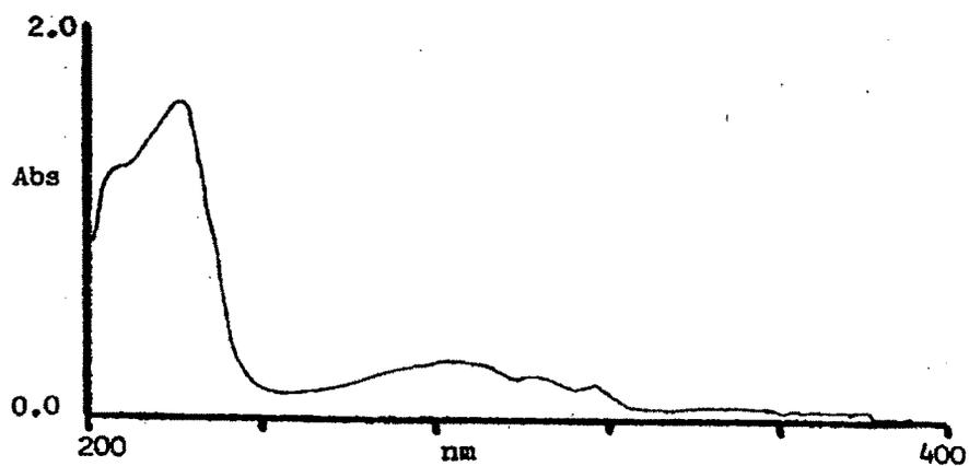
**Table 3.14 Optical characteristics for mefloquine hydrochloride in PBS**
