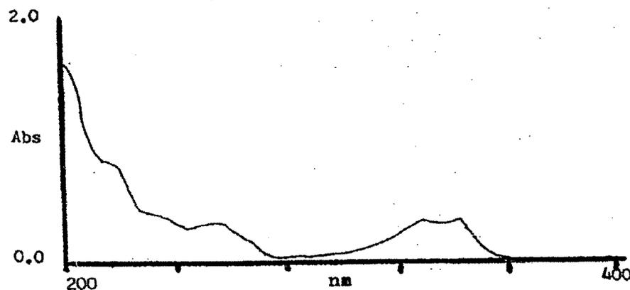
**Table 3.8 Optical characteristics for chloroquine phosphate extracted from rat blood, liver, heart, kidney & spleen into 0.01N hydrochloric acid.**
