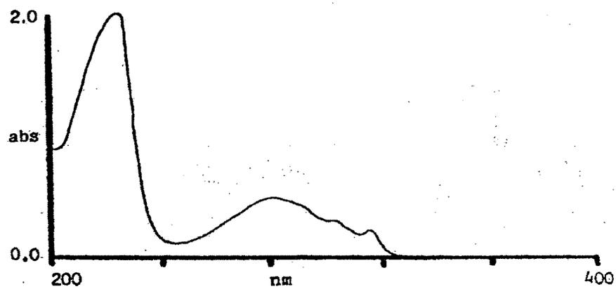
**Table 3.11 Optical characteristics for mefloquine hydrochloride in methanol**
