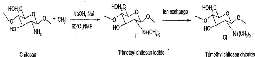
**Figure 4.4: Synthesis of trimethyl chitosan**
