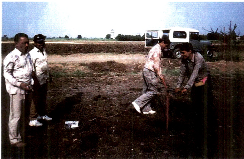
Plate VII 2 Disturbed Soil Sampling Using Standard Auguring Technique.
