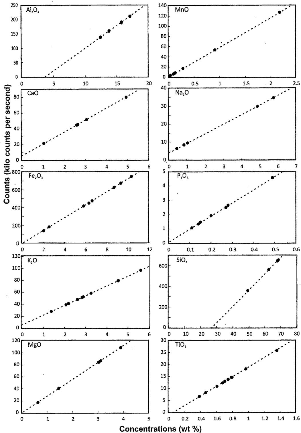
Fig. 2.9: Typical calibration curves for various major element oxides generated on XRF using multiple international rock standards.
