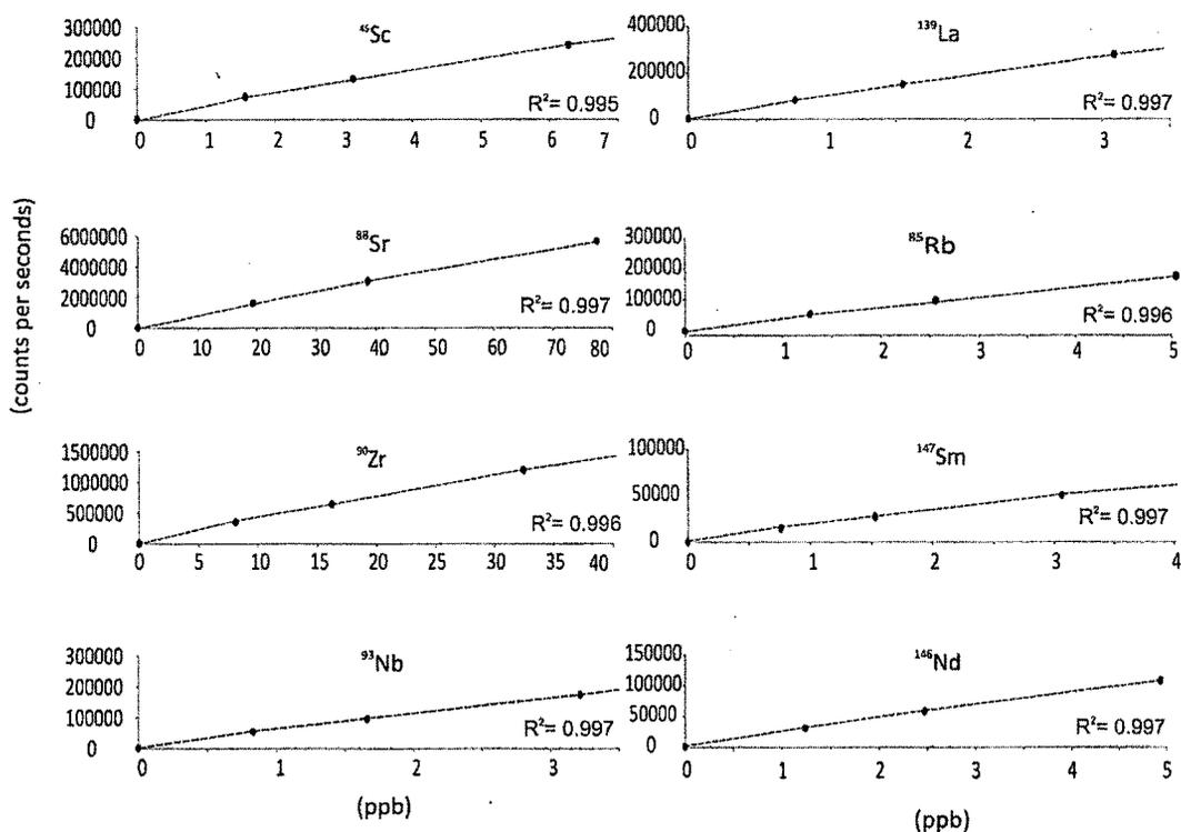
Fig. 2.10: Typical calibration curves for different trace elements generated on ICP-MS using various dilutions of BHVO-2.
