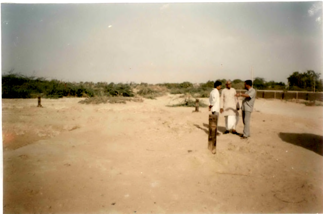
Plate 8.2 A view of piezometer nest at Santalpur
