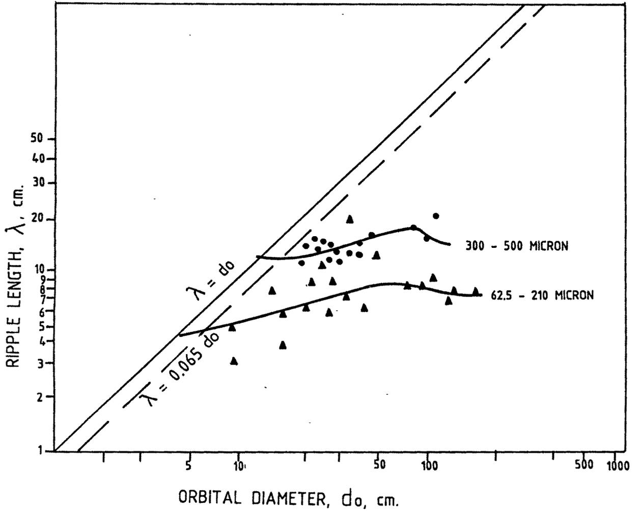
RIPPLE SPACING VERSCES ORBITAL DIAMETER IN
