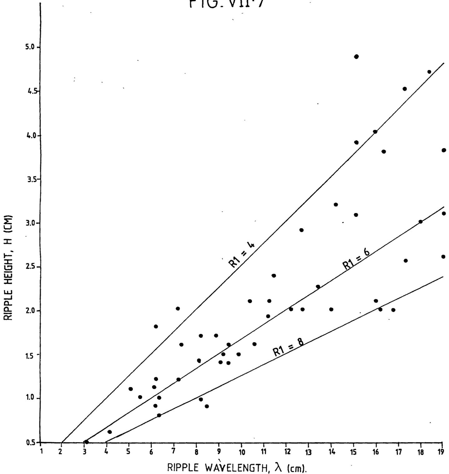
CORRELATION BETWEEN THE WAVELENGTH AND HEIGHT OF WAVE RIPPLES OF DAHANU-KORA COAST WITH THE VERTICAL FORM-INDEX ( $\lambda/H$ ) AS A PARAMETER
