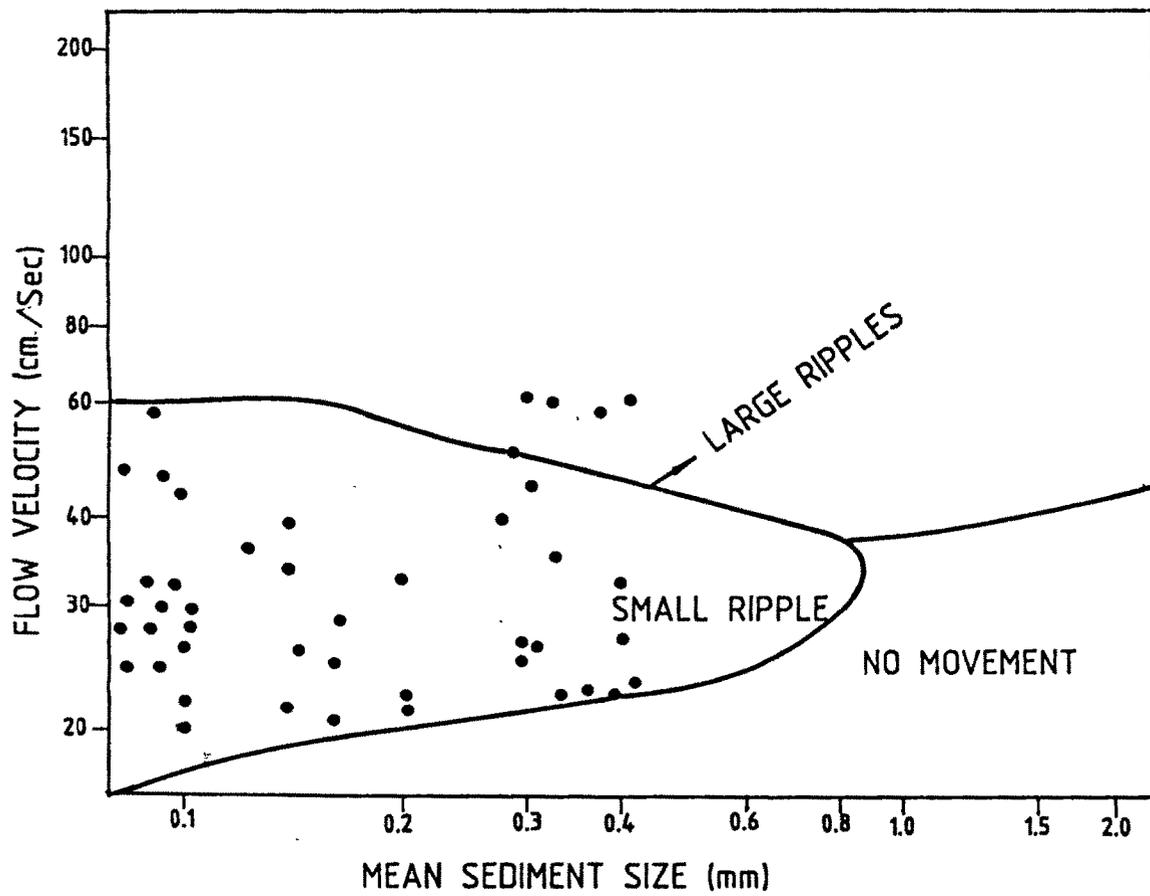
CONTROLS OF RIPPLE FORMATION BY MEAN SEDIMENT SIZE AND VELOCITY OF FLOW FOR A CONSTANT DEPTH OF FLOW.
