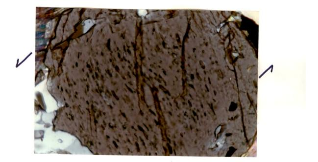
Plate-III.34 Rotated garnet. Inclusions of quartz are perpendicular to the main foliation. The rotation of garnet porphyroblast is sinistrally observed. (M : 20x at 45° cross nical position).
