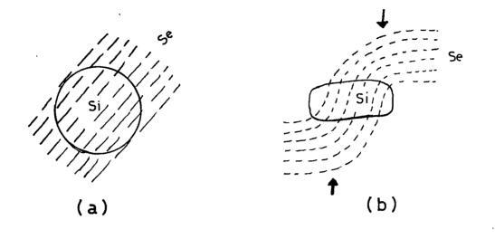
Figure III.12 Rotation of S with respect to stationary S due to coaxial deformation.
