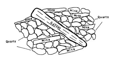
Figure III.13 Microscopic sketch showing stretched garnet porphyroblast splitting the mica flakes in garnet-mica-schist.
