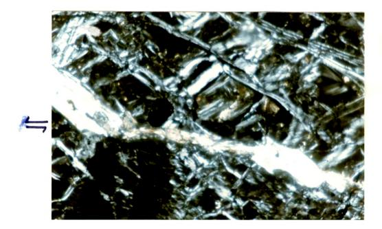
Plate-III.27b Antithetically detached mica-fish in serpentinites. The shear plane has also been serpentinized. The sense of movement is sinistral. (M = 20X, PPL).
