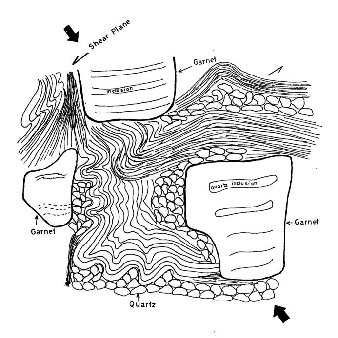
Figure III.10 Microscopic sketch showing sinistral shear sense locally developed due to pure shear deformation which later on changed into simple shear. This is few of such features survived after the area has undergone simple shear deformation.
