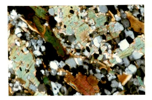
Plate-III.28 Antithetic splitting or pull-apart structure of mica grain. Space created is filled by quartz grains. The grain is sinistrally sheared. (M-20X XN)
