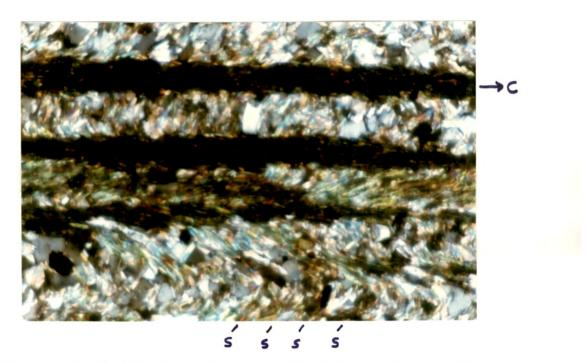
Plate-III.26 Mylonites showing S-C fabrics in the shear zone running through the non-garnetiferous schists. (Magnification - 20x, XN position).
