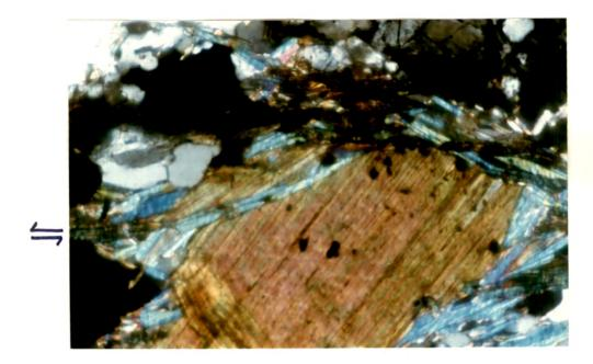
Plate-III.27a Formation of mica-fish by micro-faulting or microshearing from pre-existing mica-grain. The mica-fish shows sinistral sense of movement (M- 20x, XN)
