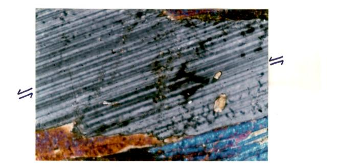
Plate-III.30a Here plagiclase grain is synthetically sheared showing sinistral sense of movement.(M-20x, XN)
