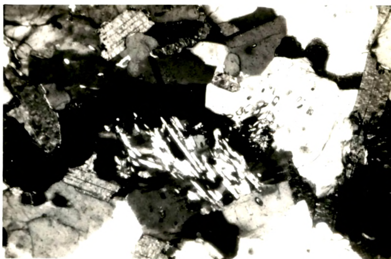
Cordierite in pelitic granulites showing pinitization along cracks. (Photomicrograph. Crossed nicols. X 80)
