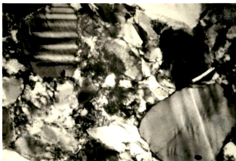
Photomicrograph of a typical non pebbly sub-graywacke. (cross nicols, X80).
