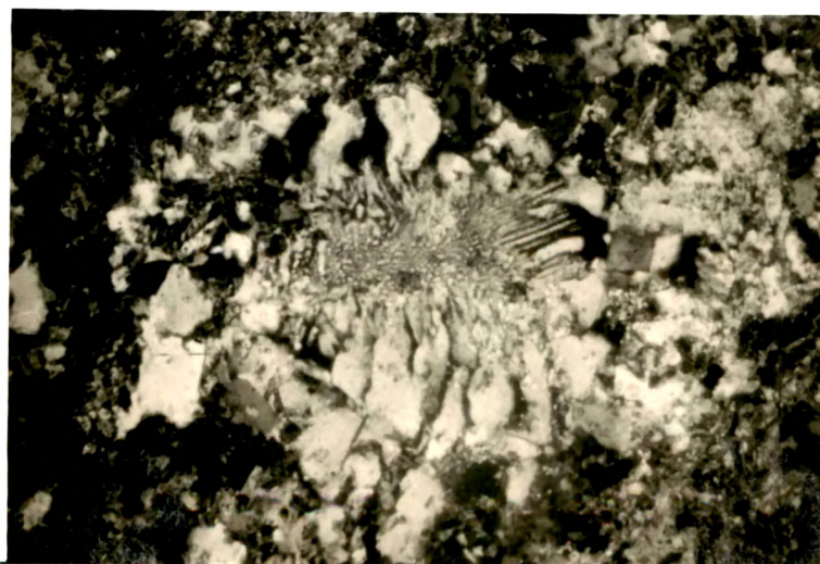
Photomicrograph of unsheared granophyre showing typical quartz-feldspar intergrowth (cross nicols, X80).
