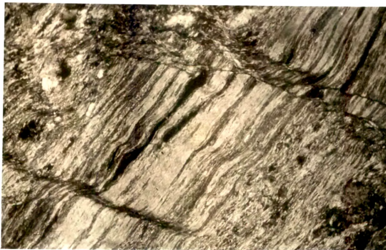
Sheared granitic rock showing crenulation cleavage. (Photomicrograph: cross nicols, X45).
