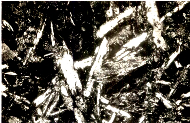
Coarse basaltic texture of traps (Photomicrograph: cross nicols, X45)
