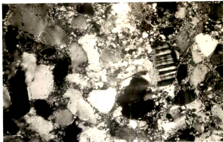
Heterogeneous coarse matrix (sub-greywacke) of Blaini bouldary beds (Photomicrograph: cross nicols, X45).
