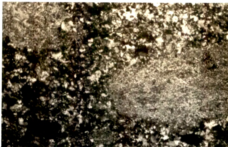
Sheared granitic rock showing granulation and alteration of feldspars. (Photomicrograph: cross nicols, X45).
