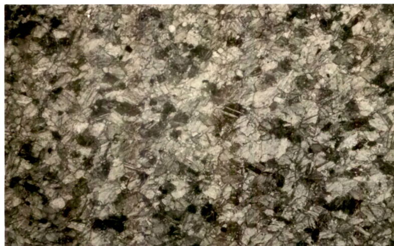
Texture of Blaini limestone (Photomicrograph: polarised light, X45)
