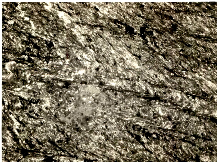
Crinkled phyllonites with a strain-slip cleavage. (Photomicrograph: Crossed Nicols X80)
