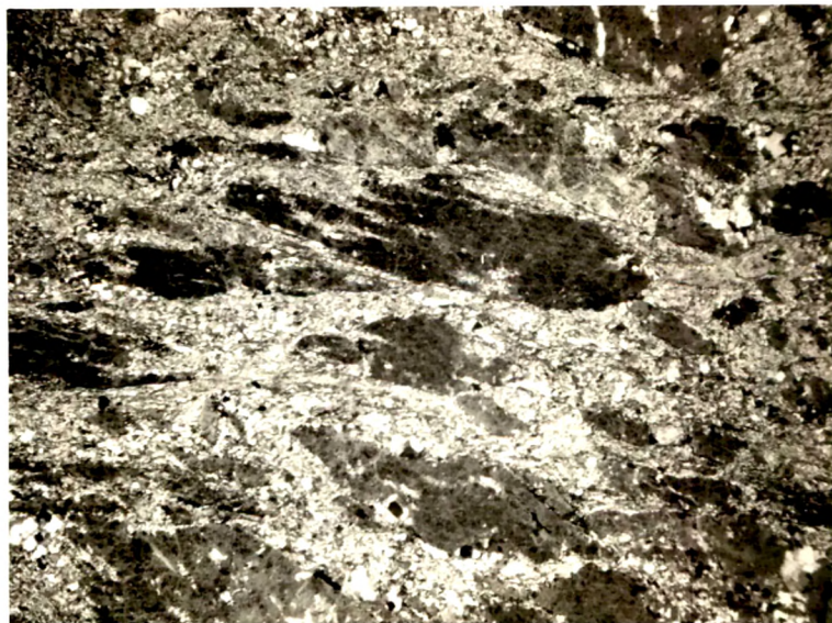
Altered and drawn out relict of feldspar in mylonitised gneiss. (Photomicrograph; Crossed Nicols X30)
