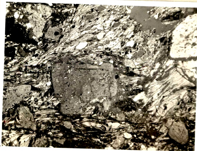
Texture of a partly mylonitised gneiss showing an advance stage of crushing and granulation. (Photomicrograph: Crossed Nicols X30)
