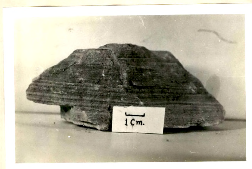
Parallel lamination in Sandstone Overlying fireclay.
