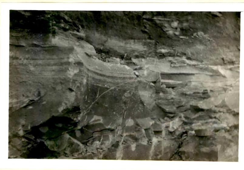
Flinty fractures and color banding in fireclay.
