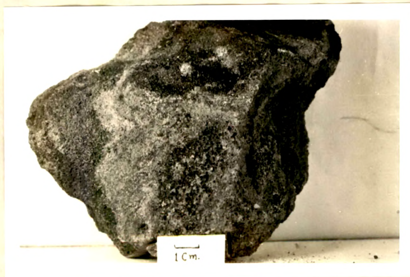
Iron concretions in ferruginous sandstone of Upper Dhrangadhra Formation
