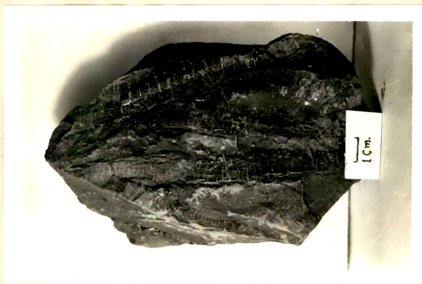
Coaly matter (Plant impressions) on upper layer of fireclay bed.
