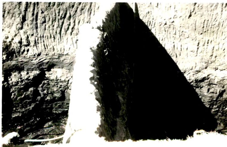
The boundary wall between the adjacent mining pits is less than 0.5m. which is not in conformation to mining laws.
