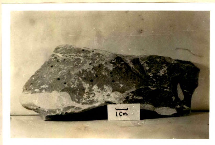
Iron concretions in fireclay (flint clay)
