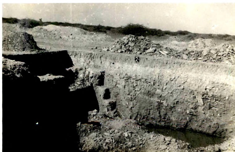
Mine pit showing 6m. thick semi-flint clays and water flooding.
