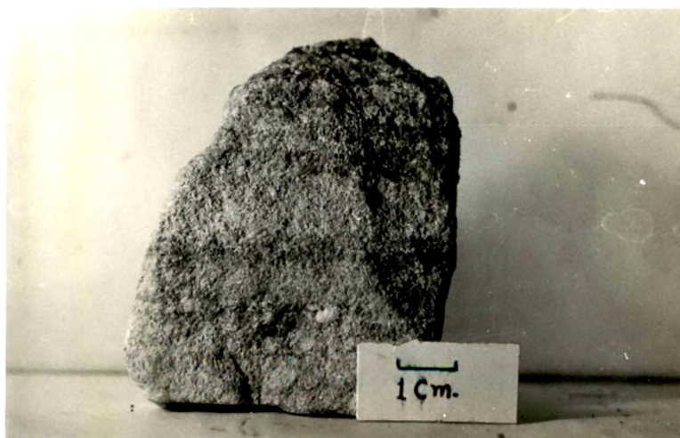
Graded bedding in sandstone overlying fireclay.
