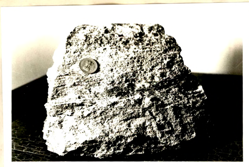
Plate I. Graphite schist showing alternate grayish brown and light yellowish bands (Ankli).
