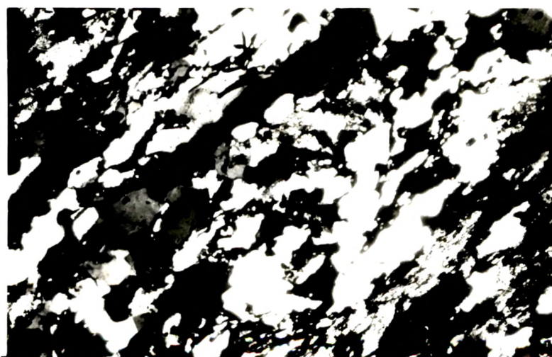
Plate XXIVB. Graphite schist (Ankli) showing graphite flakes disseminated in light whitish yellow band (Photomicrograph: Polarized light, X60).
