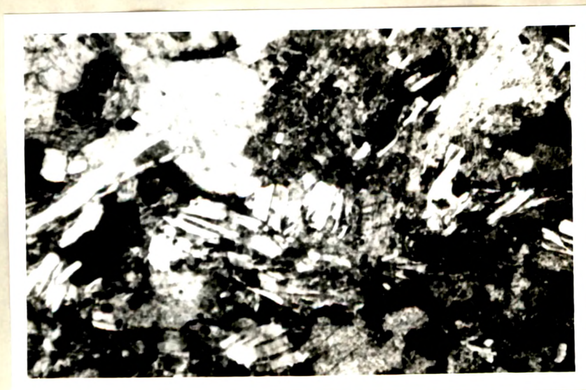
Plate XXVI. Crystalline limestone (Ankli) showing presence of tremolite (Photomicrograph: Crossed nicols, X60).
