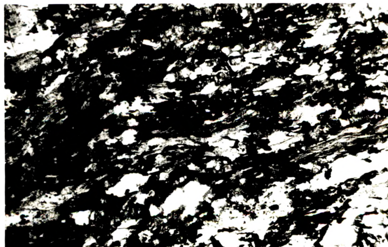
Plate XXIIIB. Graphite schist (Ankli) showing graphite flakes disseminated in grayish-brown band (Photomicrograph: Polarised light, X60).
