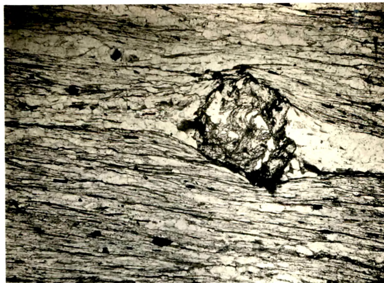
Rotated garnet in mica schist. (Photomicrograph X30)
