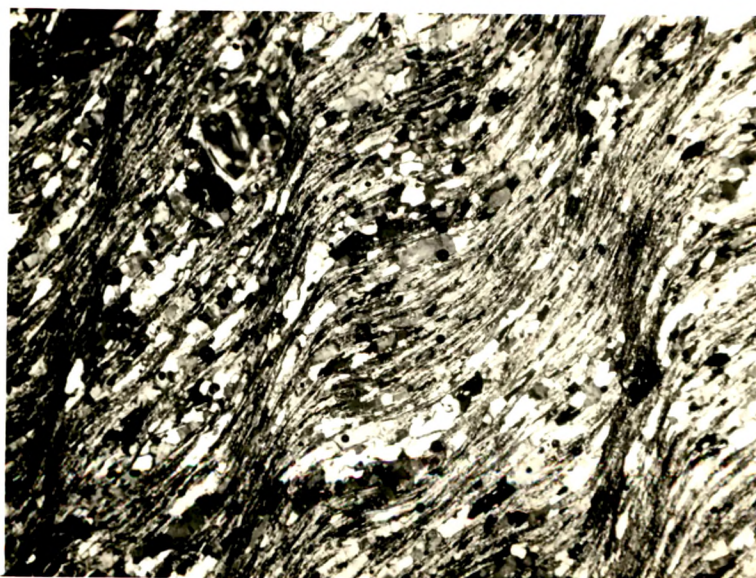
Crinkling due to differential slipping in Nathuakhan phyllites. (Photomicrograph X30)
