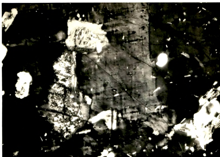
Porphyroblast of potash feldspar showing super- imposition of cross hatching over carlsbad twins. (Photomicrograph X60)
