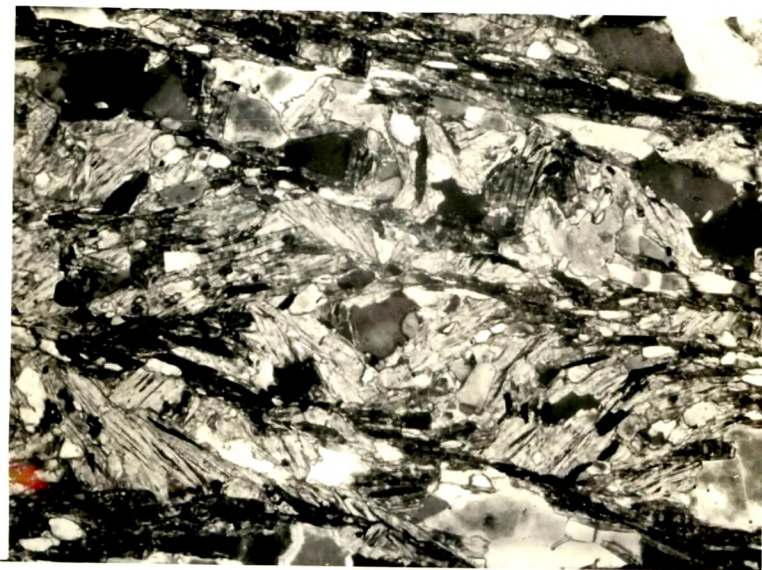
New micas along fractured hinges of microfolds. (Photomicrograph X60)
