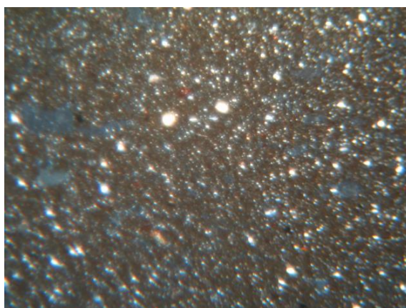
Figure 4.97: Photomicrograph of a Turquoise Glazed Ware (sample no. S-TGP 3) from Sanjan in Cross Polarised Light (XPL) with a micaceous matrix and highly fine and well sorted quartz petro-fabric. Petro-Fabric Group 12. Field of view: 0.18 mm 2
