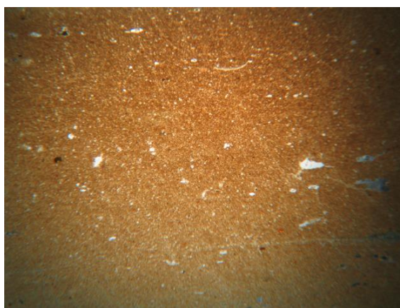
Figure 4.88: Photomicrograph of a Sgraffiato Ware S-LS4 in Plain Polarised Light (PPL). Petro-Fabric Group 8a. Field of view: 0.18 mm 2
