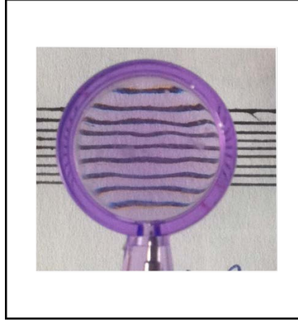
Fig 3.1 Recorded modulation of line pattern projected through a lens.
