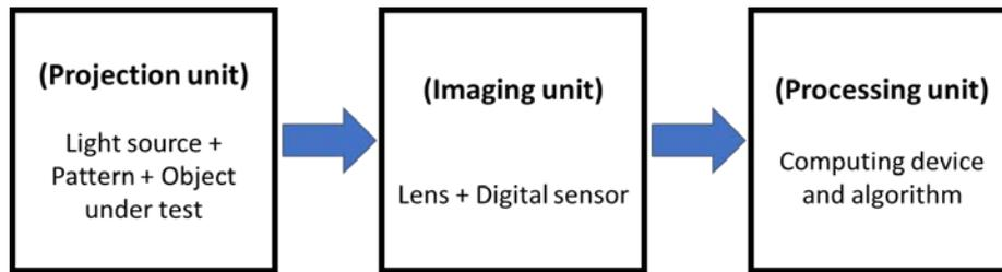
Fig 1. 4 Block diagram of Fringe projection technique
