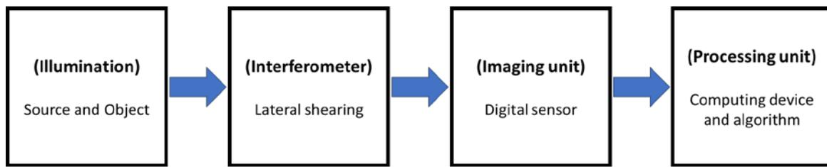
Fig 1. 5 Block diagram of Lens-less digital holographic technique
