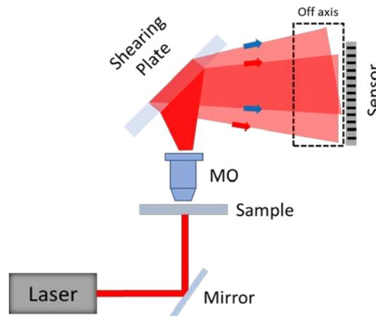
Fig 1. 3 Schematic of Lateral shearing geometry
