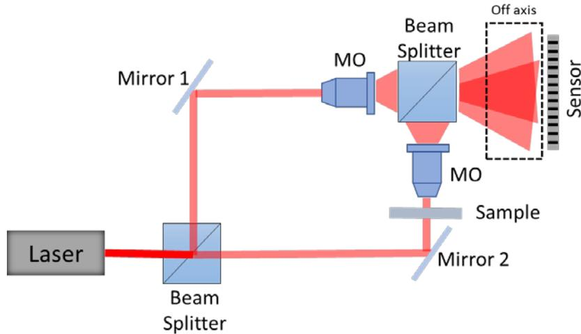
Fig 1. 2 schematic of Mach-Zehnder interferometer configuration for digital holographic microscopy
