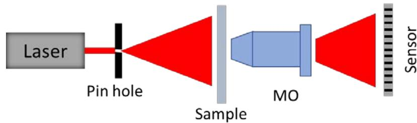
Fig 1. 1 Schematic of in-line digital holography configuration
