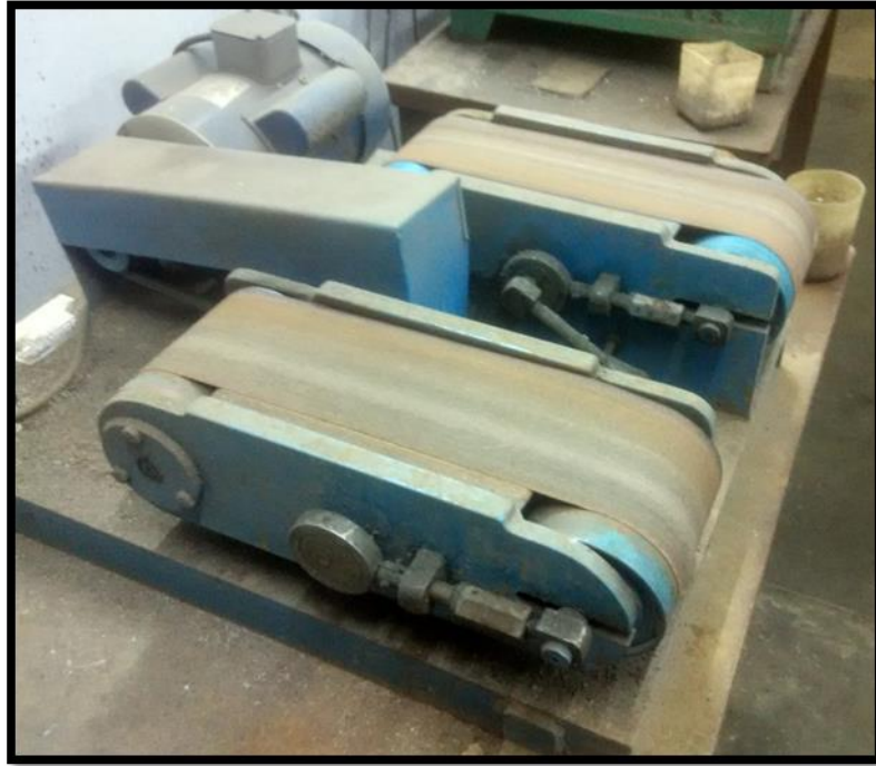
Fig. 3.11: Belt Polisher used for Rough Grinding
