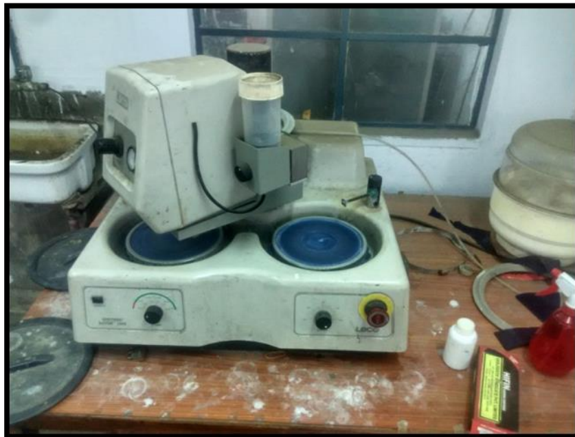
Fig. 3.12: Wheel Polisher Used for Fine Polishing
