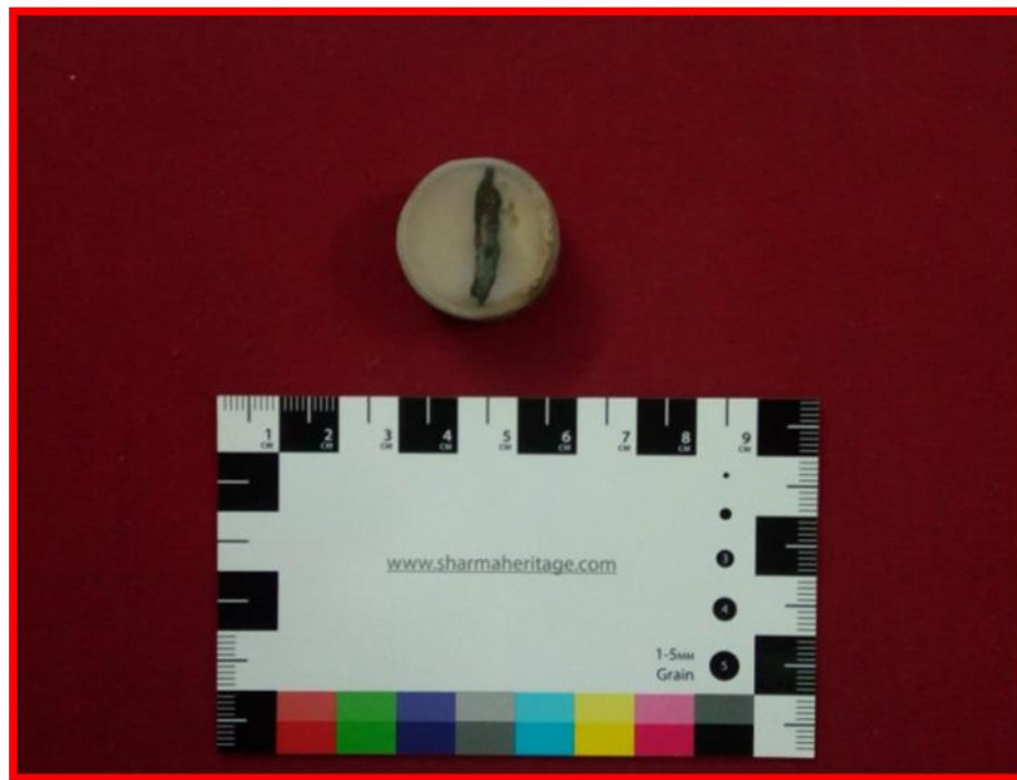
Fig. 3.10: Plastic Mounted Specimen Ready for Microscopic Viewing
