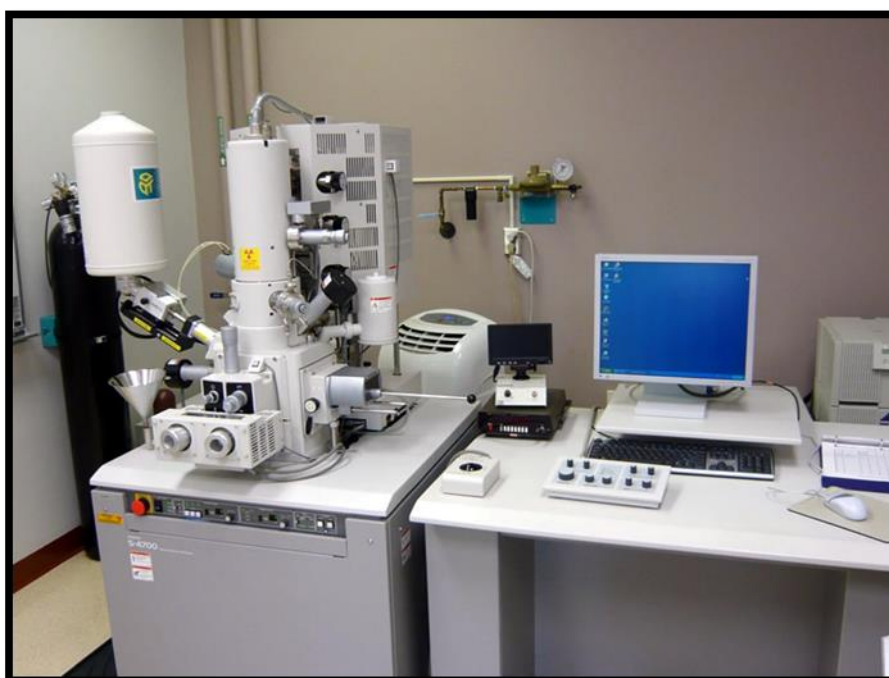
Fig. 3.15: Scanning Electron Microscope Coupled with Energy Dispersive X-Ray Spectrometry
