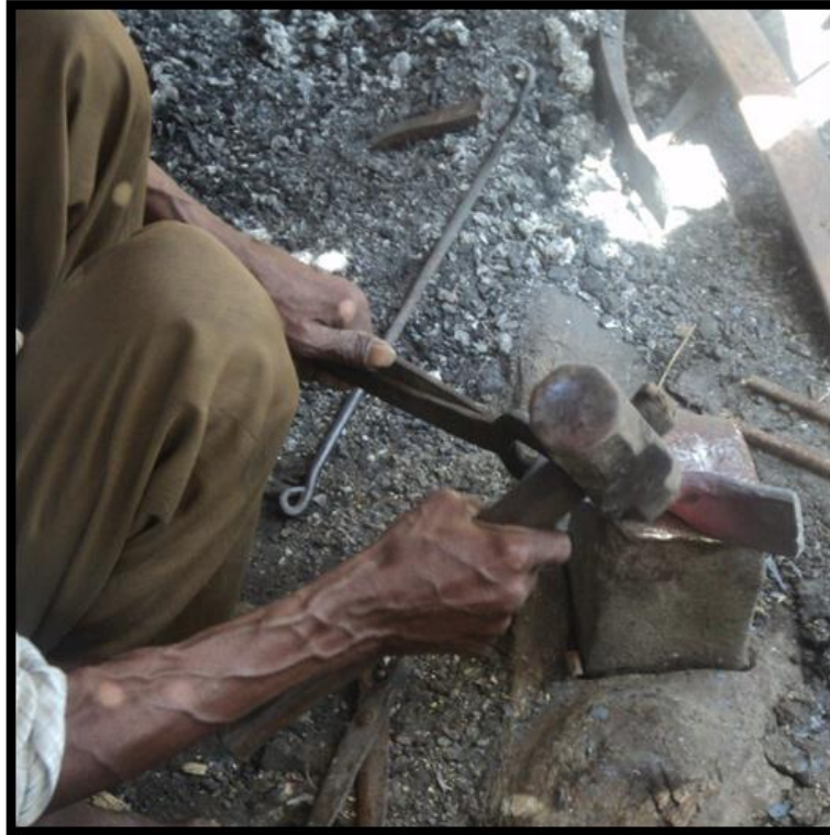
Fig.4.6.1.5.3.g: Detached Segment B Forged in Red-Hot Condition
