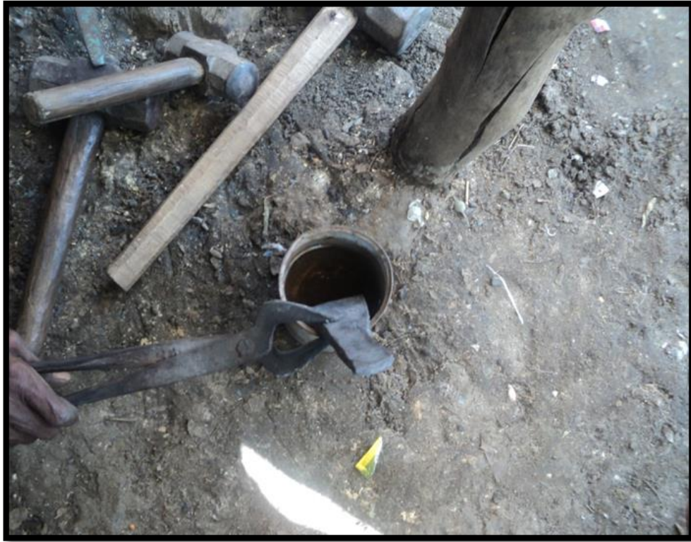
Fig.4.6.1.5.3.1: Quenching of Section C
