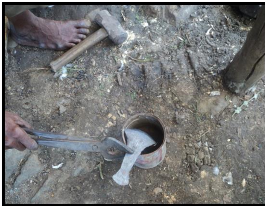
Fig.4.6.1.5.1.d: Quenching of the Broader Blade
