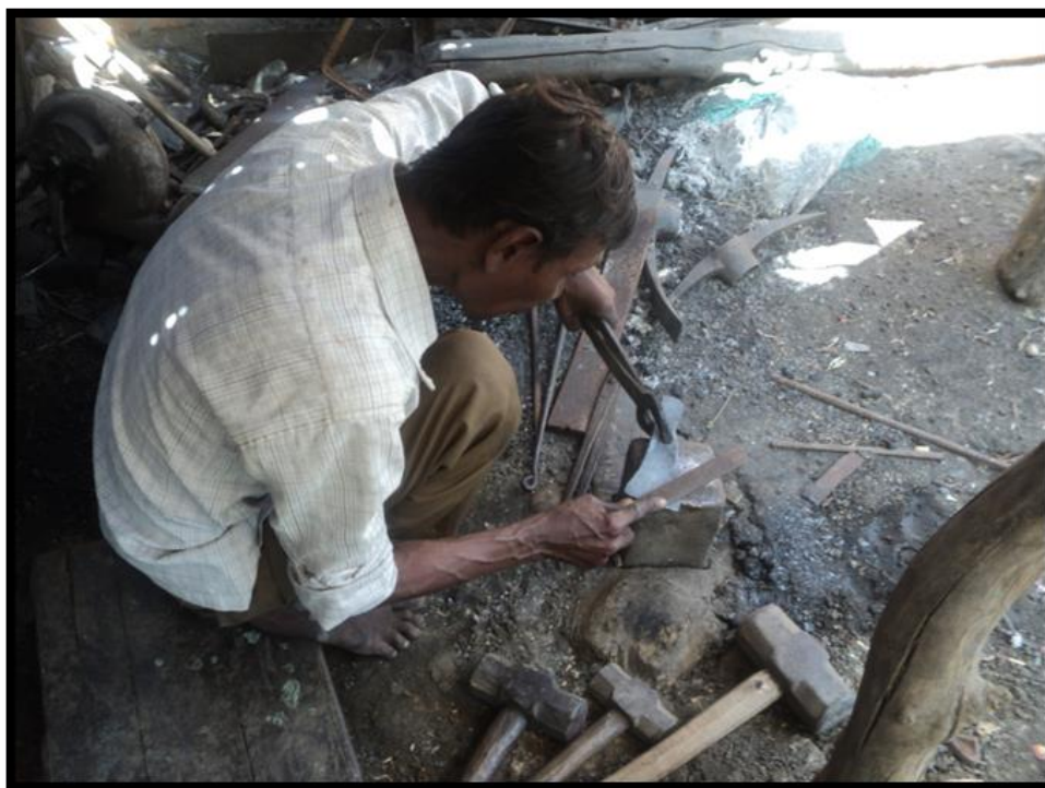
Fig.4.6.1.5.3.k: Sharpening of Cutting Edge (C)
