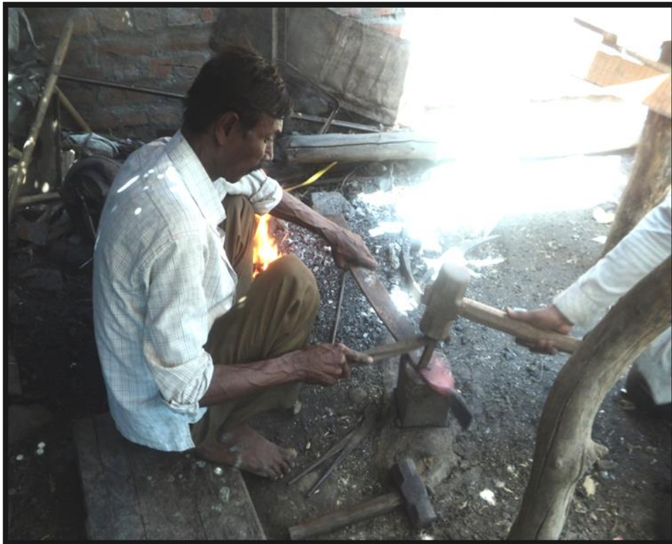
Fig.4.6.1.5.3.e: Detachment of Segment B Using a Chisel
