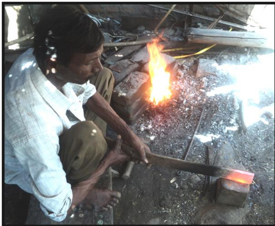
Fig.4.6.1.5.3.c: Segment B in Red-Hot Condition
