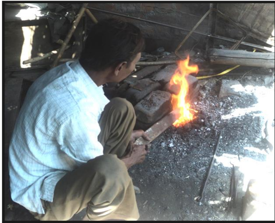
Fig.4.6.1.5.3.b: Annealing in Process
