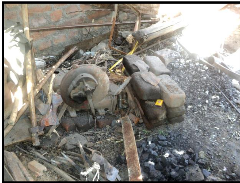
Fig. 4.6.1.4.b Blower Attached to the Brick Furnace
