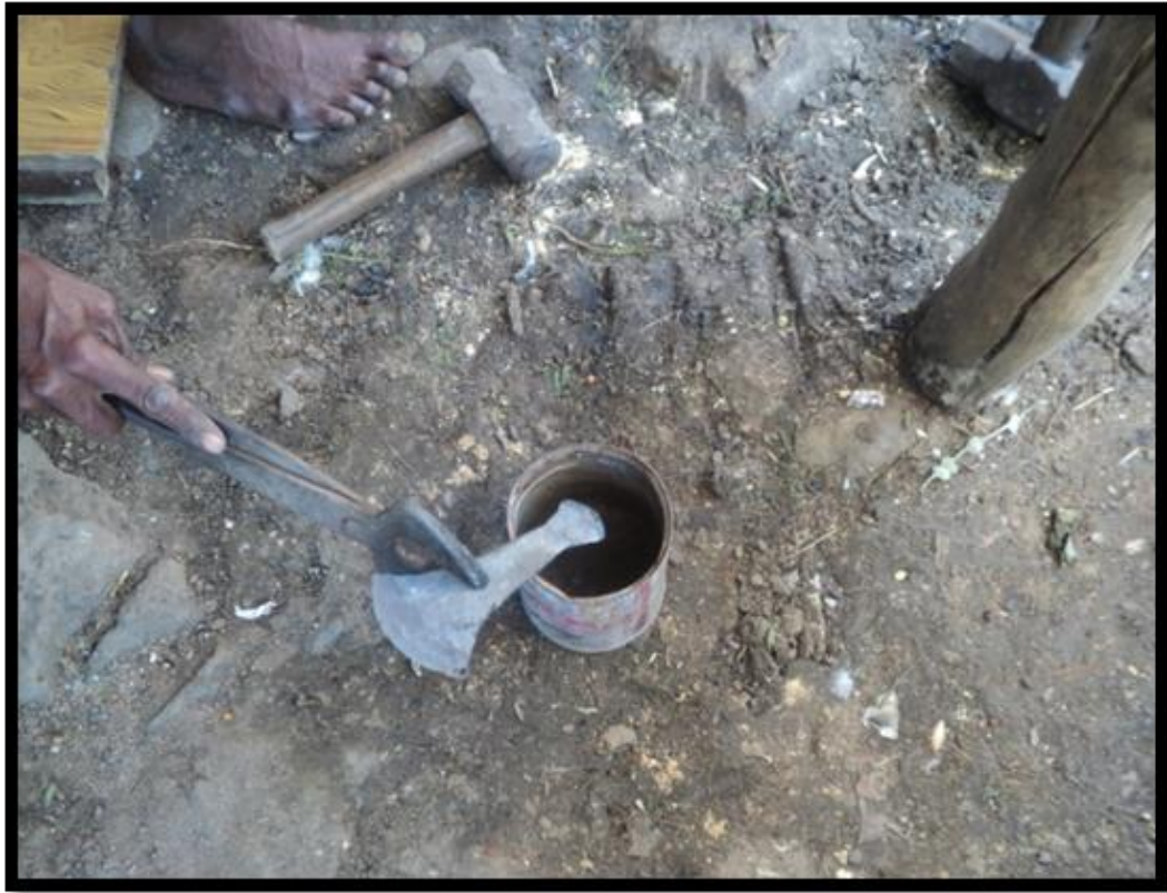
Fig.4.6.1.5.1.e: Quenching of the Narrower Blade
