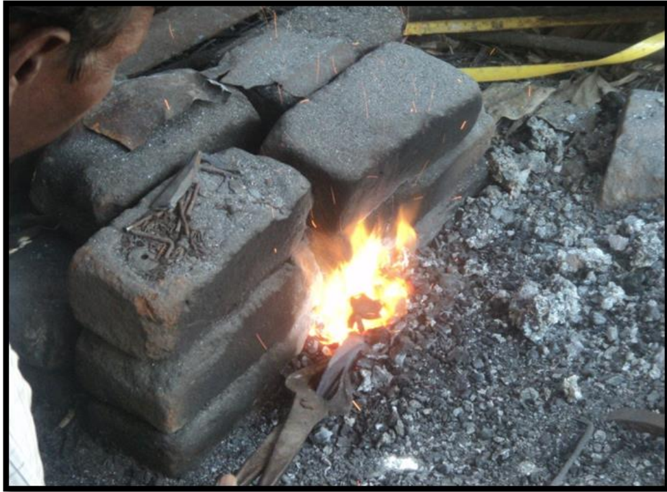
Fig.4.6.1.5.3.h: Annealing of Butt End for the Folding Process
