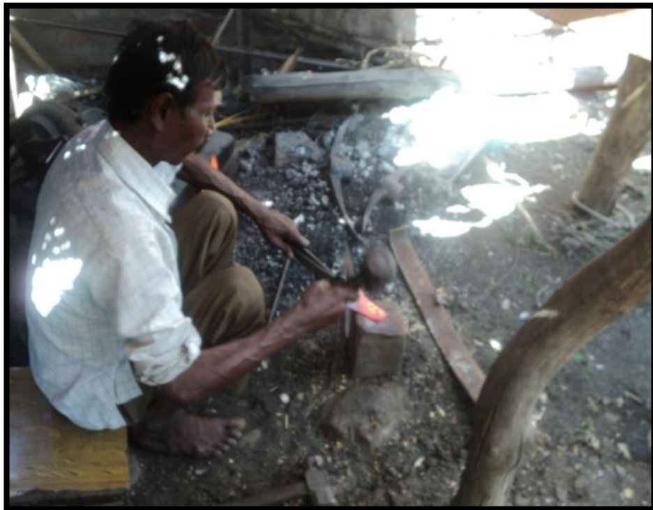
Fig.4.6.1.5.1.b: Cut Shape Being Forged in Red-Hot
