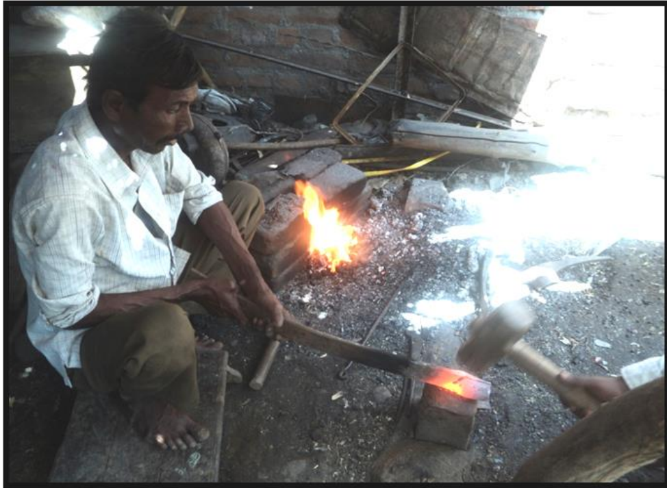
Fig.4.6.1.5.3.d: Forging of Segment B in Red-Hot Condition
