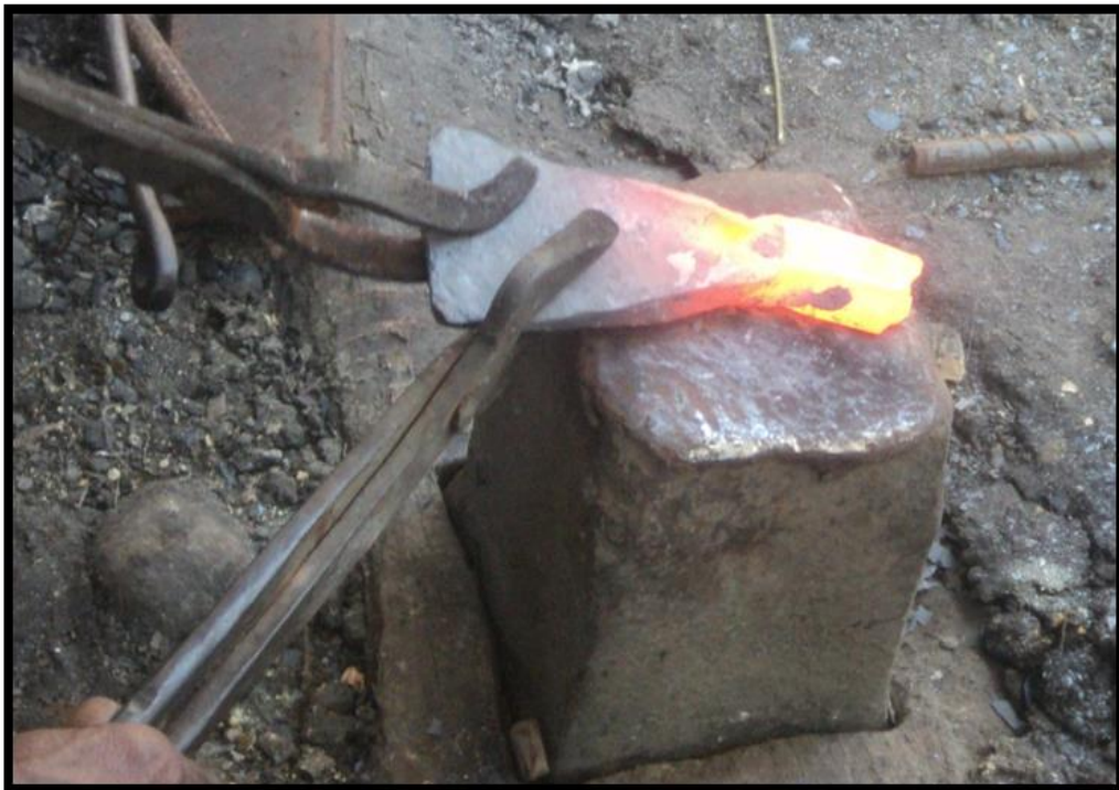
Fig.4.6.1.5.3.i: Butt End in Red-Hot Condition
