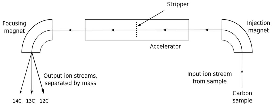
**Figure 3.7** Demonstration of a complete working model of Accelerator mass spectroscopy used for radiocarbon dating.
