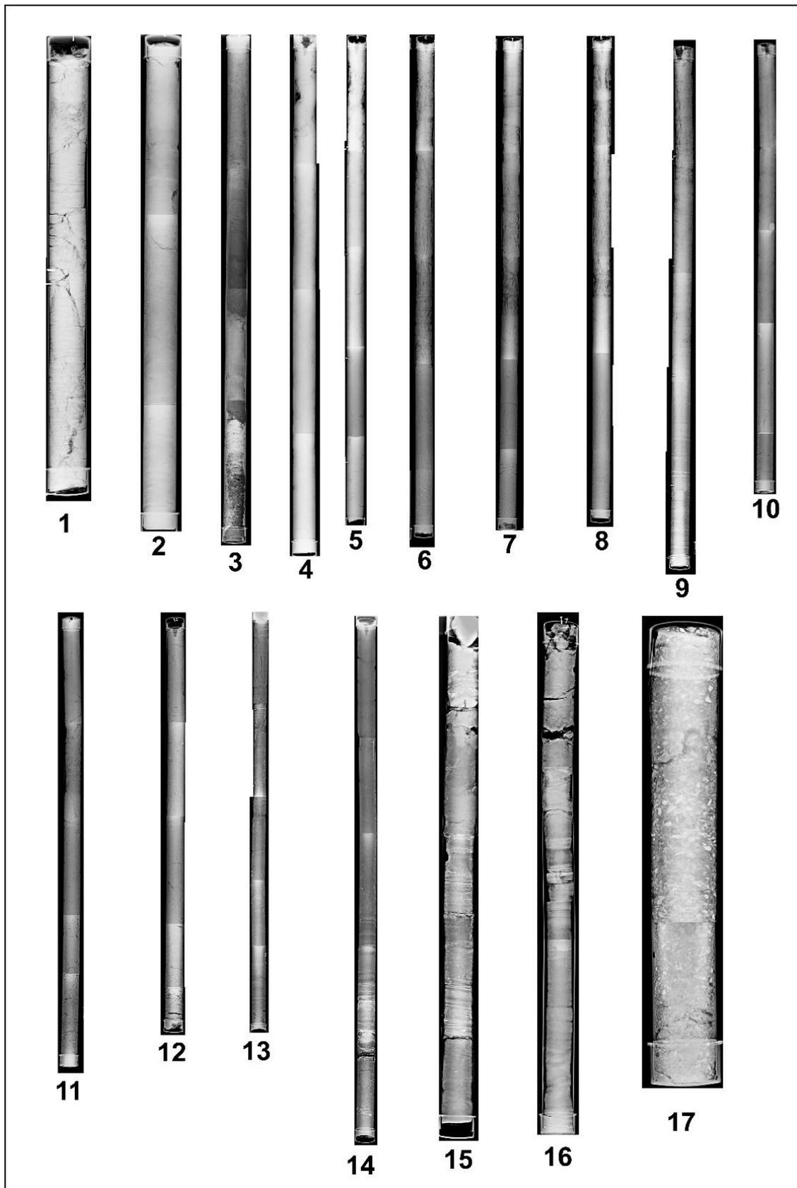
**Figure 3.3** X-Ray radiographs of all core pipes from the Berada core location. Note the excellent core recovery and fine-scale laminations in the core pipes.
