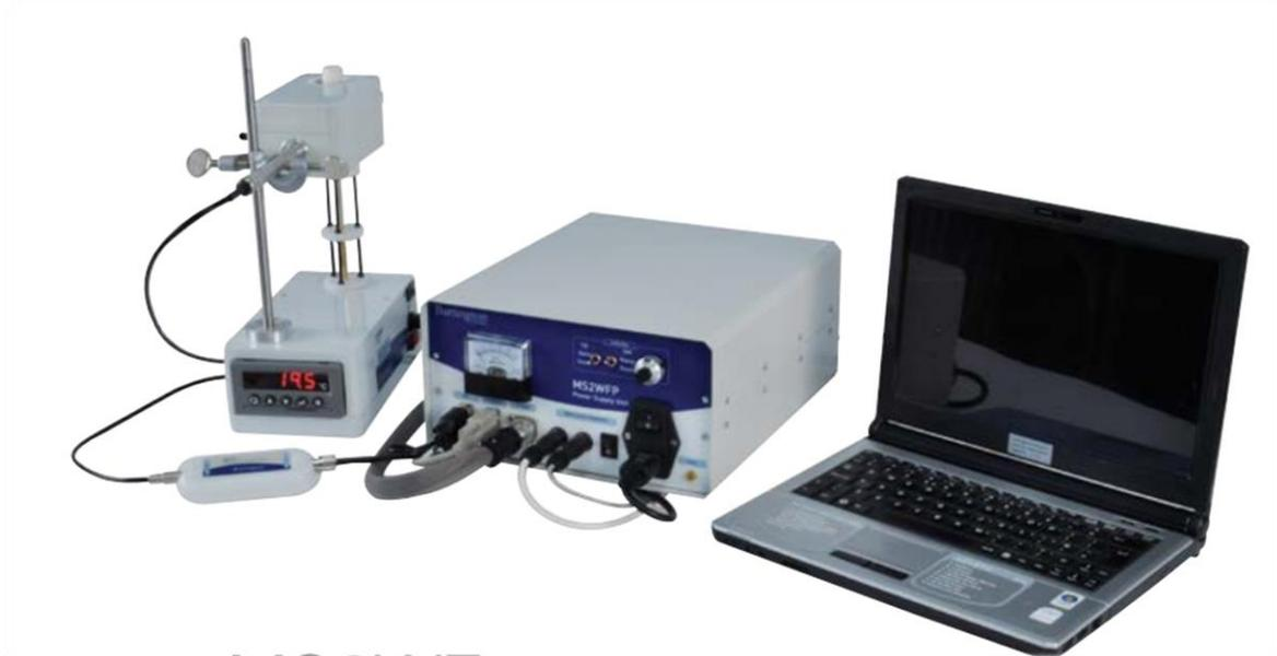
**Figure 3.4** Bartington MS2WFP Susceptibility Meter (noise level  $\sim 3 \times 10^{-9} \text{ m}^3 \text{ kg}^{-1}$  for a 10 g sample). The instrument is used to calculate concentration of magnetic mineral.
