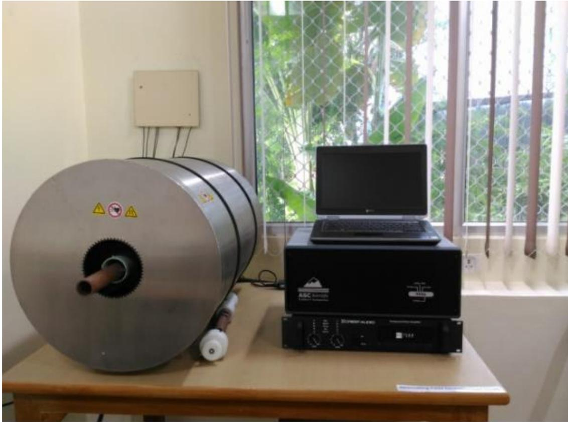
**Figure 3.6** ASC Scientific D2000 Alternating Field Demagnetizer.
