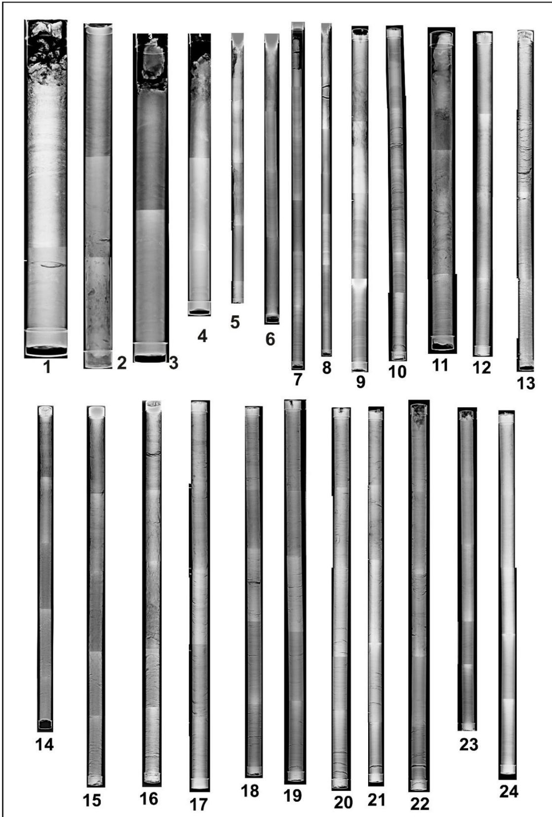
**Figure 3.2** X-Ray radiographs of all core pipes from the Dhordo Core site. Note the excellent core recovery and fine-scale laminations in the core pipes.
