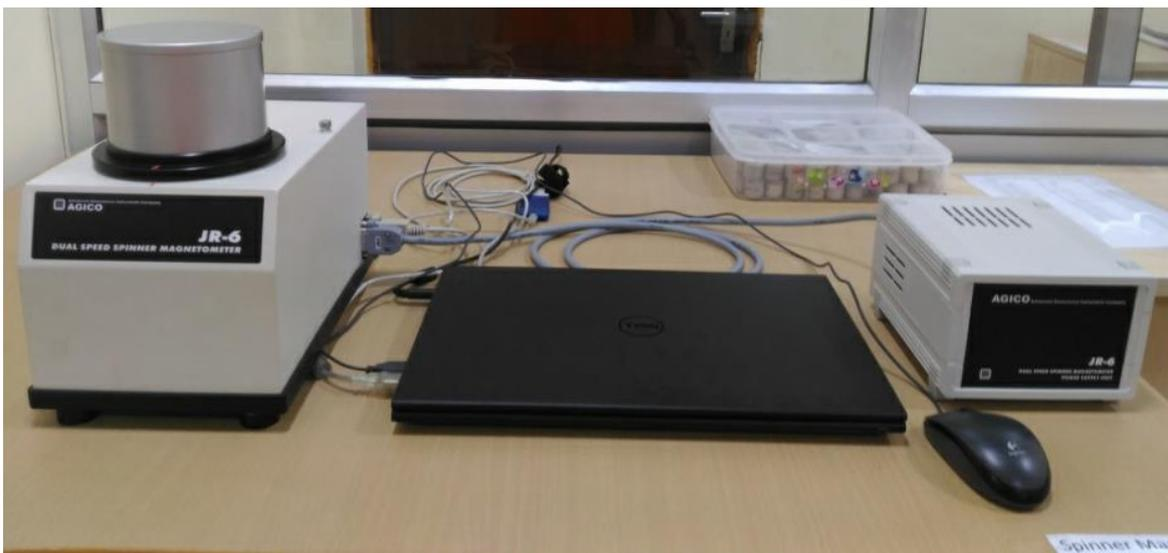
**Figure 3.5** AGICO JR-6 Spinner Magnetometer (JR-6 Dual Speed Spinner Magnetometer) Measurement over 11 magnitudes ( $10^6 - 10^4 \text{ A/m}$ ).
