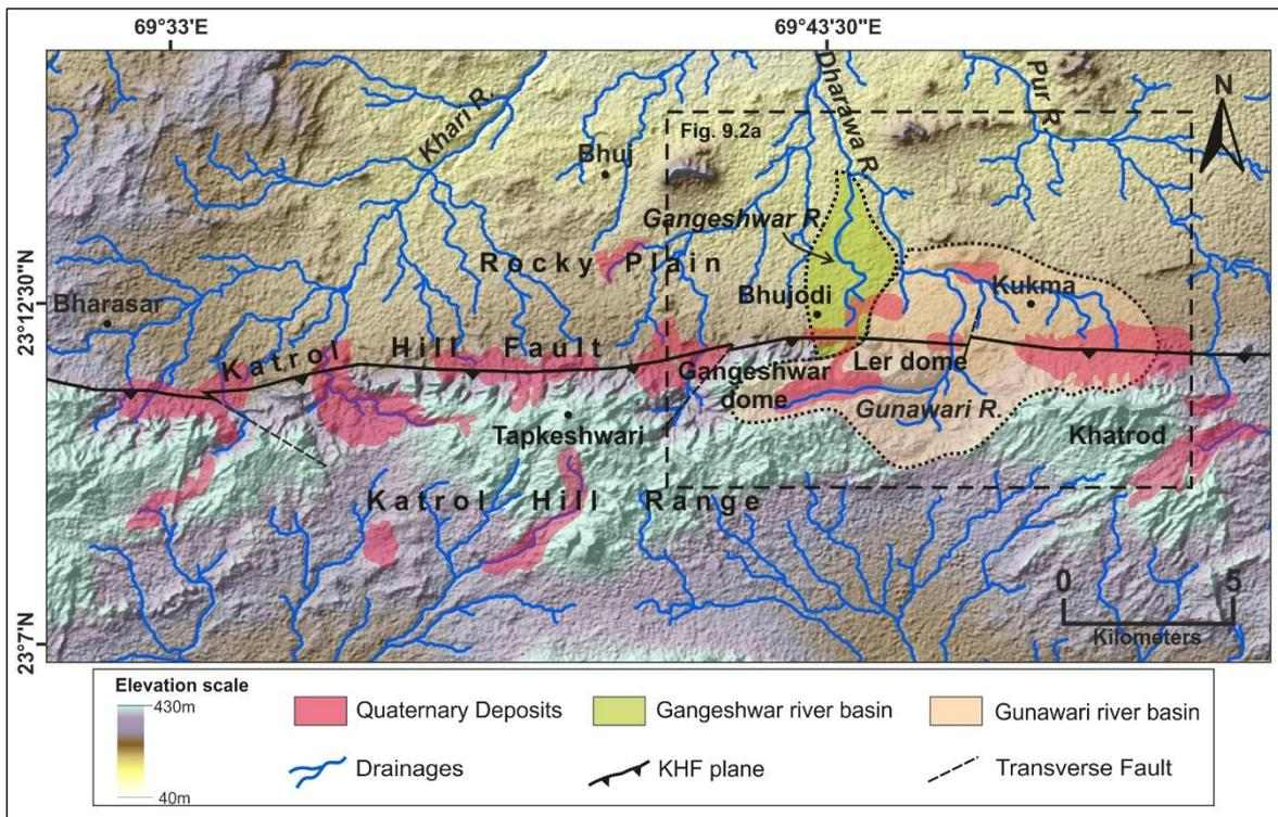
**Figure 9.1** DEM of Katrol Hill Fault (KHF) zone (modified after Patidar et al., 2008). Note the rugged hilly topography of the Katrol Hill Range bounded by the KHF in the north. Also seen are the north and south-flowing drainage lines. Boxed area in dashed lines show the area covered in Figure 9.2a. Red colour indicates Late Quaternary miliolite deposits.
