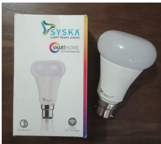
Plate 2: Syska Smart Pumpkin Wi-Fi 9W Bulb 3 in 1 color (3000k-4000k-6500k) used for the study
