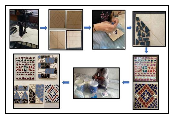
Plate 8: Process of making Kitchen Tiles
