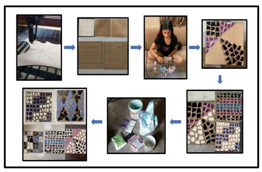
Plates for the Process of making Ceramic Waste Tiles
