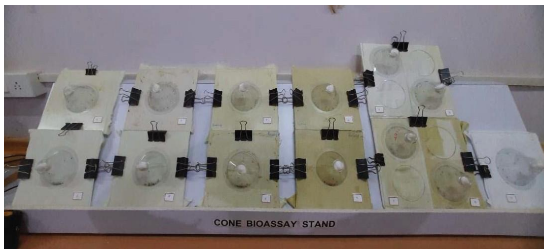
Plate 3.14: Cone test of all finished fabric to evaluate mosquito repellency
