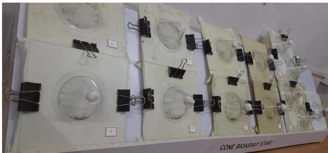
Plate 4.5: Cone test for evaluate mosquito repellency of treated fabric
