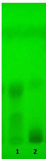
Figure 3.12a Tracks: 1. Precipitates from ethyl acetate fraction; 2, purified swertisin, visualization UV 254 nm
