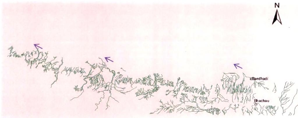
**Fig. 4.7:** Drainage map of the area along Kachchh Mainland Fault showing the deflection of the streams towards west.
