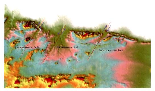
Fig.6.8: Strike-slip movement along the Lodai, Pur and Kaila transverse faults visible on the DEM of the area along KMF.
